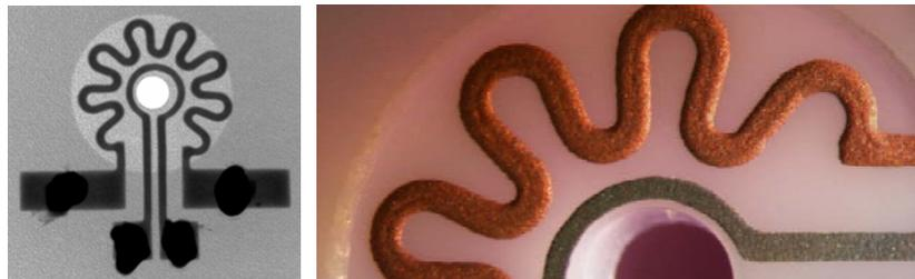
**Figure 3.** X-ray image of full-fledged combustor with a combined heater and oxygen supply meandering around the circular temperature sensor, inside which the sample inlet and gas outlet combine to make a bright circle (left), and microscope close-up of open reactor just after copper plating of the heater, not having affected the platinum temperature sensor (right).
