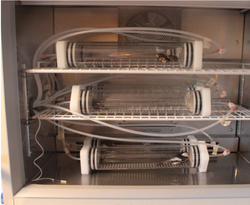
Figure 2: Respirometry tubes for measuring resting metabolic rate of flycatchers on Öland. We had eight tubes, where one tube was always empty to act as baseline, to measure up to seven birds at one time.
