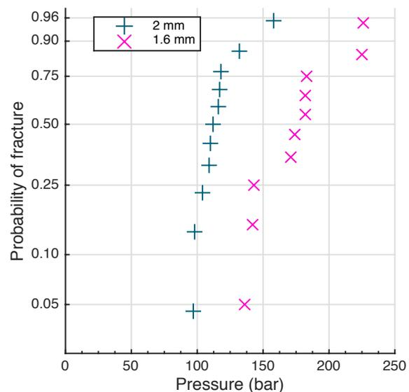
**Figure 3** Fracture pressures of blister test structures with two cavity diameters.
