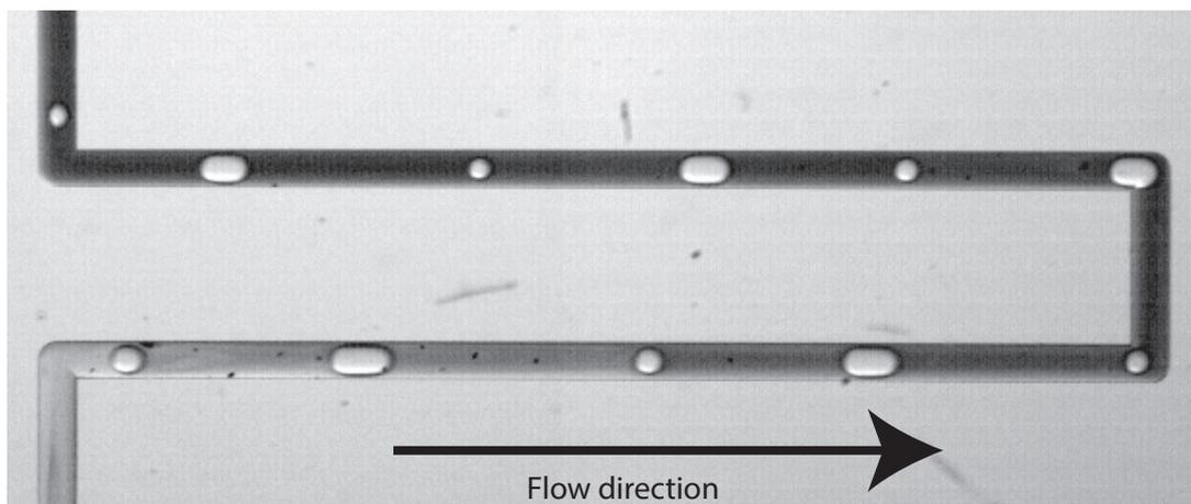
**Figure 4** High-speed image at 421 nm. Flow of segments containing high density CO<sub>2</sub> in an aqueous solution containing BPB. As time progresses, light absorption is seen in the aqueous phase indicating a pH drop.
