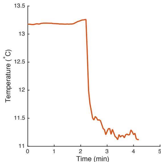
**Figure 2** Temperature drop of channel wall after adjusting system pressure from 90 to 70 bar.
