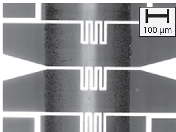
**Figure 1** Three Pt temperature sensor elements embedded in the chip and exposed to the fluid inside of the channel.
