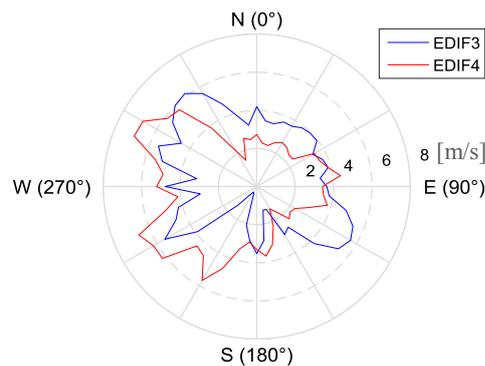
**Figure 3.** Mean wind speed of EDIF 3 and EDIF 4 building at each sector simulated
