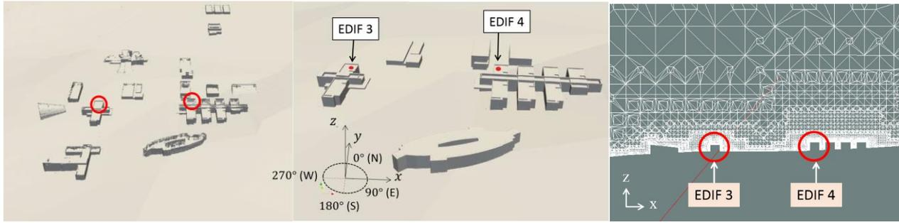
**Figure 2.** Computational mesh of building in Huesca, EDIF 3 and EDIF 4 developed in graphical user interface software
