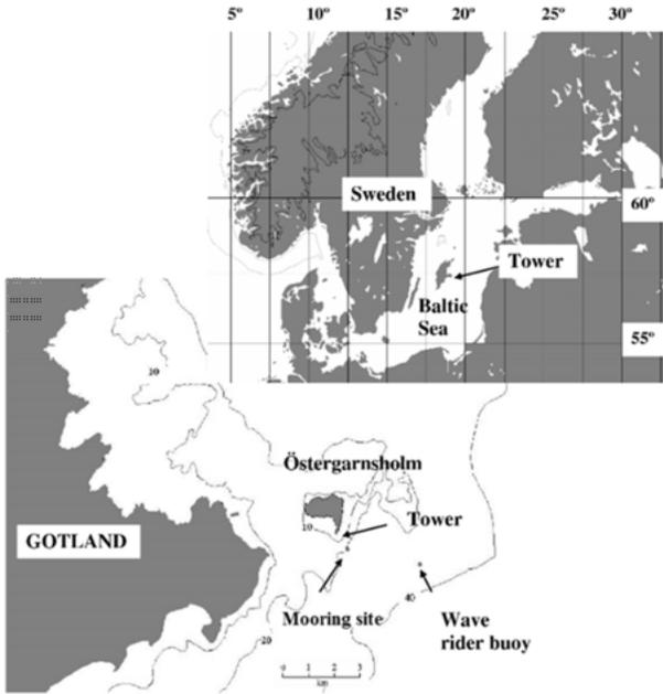
Figure 1. Map of the Östergarnsholm measurements site. Positions of the tower, mooring instruments and wave buoy are indicated by arrows. Thin solid lines represents iso-lines of water depth. (Reprint from **Paper II**)
