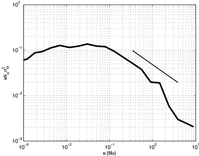
Figure 3. Normalized mean power spectra of  $O_2$  measured with the non-optical isolated  $O_2$  sensor shown against frequency. The spectra is averaged over 50 half hours of data from 29 August to 30 August 2012, at the height of 27 m. Straight solid black line indicates a  $-2/3$  slope (from **Paper I**).
