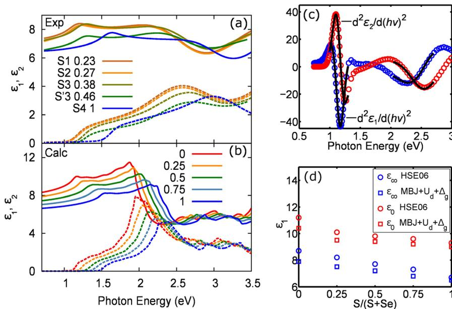
FIG. 2.  $\varepsilon_1$  (solid line) and  $\varepsilon_2$  (dashed line) determined by ellipsometry (a) and *ab initio* calculation (b), fit to  $d^2\varepsilon/d(h\nu)^2$  from critical point analysis for S1 (c), and the theory-derived  $\varepsilon_\infty, \varepsilon_0$  as a function of  $S = S/(S + \text{Se})$  (d).
