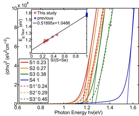
FIG. 3. Tauc plot  $(\alpha hv)^2$  v.s.  $hv$  from SE data for S1–4 and spectrophotometry data for S1'–S3' and the resulting Tauc bandgap as a function of  $x = S/(S + Se)$  in the inset.
