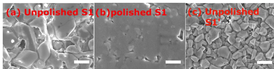
FIG. 1. SEM surface image of S1 before (a), after polishing (b), as well as S1' before polishing (c).
