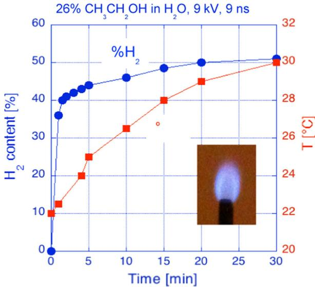
**Fig. 3** Volume of hydrogen in the produced gas and the corresponding temperature of the electrolyte versus time. The *inset* shows the picture of the flame with 50% of hydrogen in the produced gas flow of 250 sccm. The outer diameter of the nozzle with the flame is 3 mm
