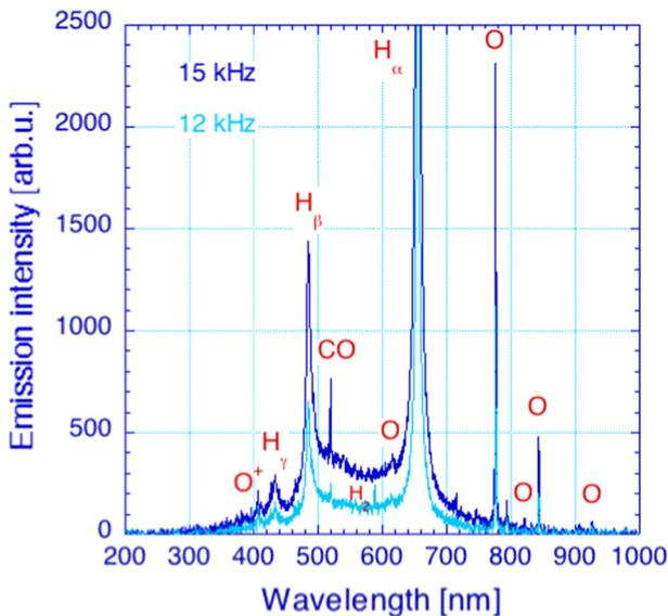
**Fig. 4** Optical emission spectra from the submerged plasma in water mixed with 26% ethanol at two repetition frequencies of the pulsed power
