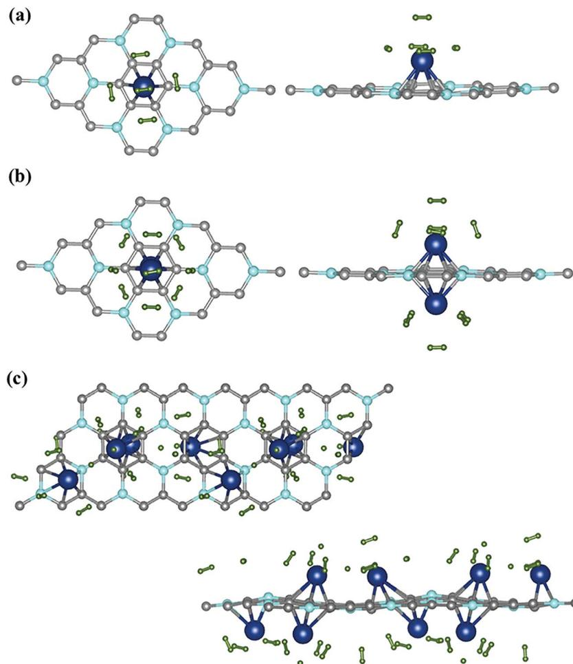
Fig. 5 Hydrogenated BC<sub>3</sub> sheets. Top view and side view for (a) 1 Sc [3.2% Sc] and (b) 2 Sc [6.4% Sc]. (c) Extended top and side view for 4 Sc [12.5% Sc].
