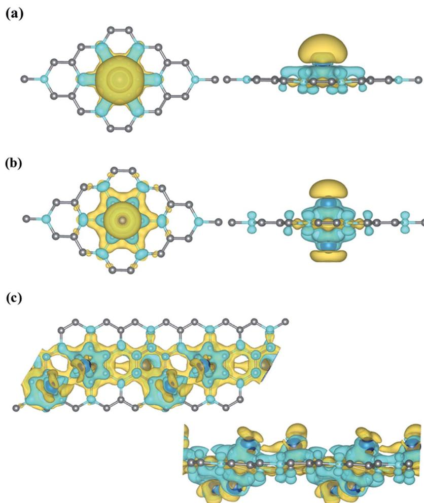
**Fig. 3** Top (left) and side (right) views of isosurface charge densities of  $\text{BC}_3$  with (a) 1 Sc atom [3.12% Sc-coverage], (b) 2 Sc [6.25% Sc-coverage] and (c) 4 Sc [12.5% Sc-coverage]. Cyan and yellow indicate the accumulation and depletion of charge, respectively.
