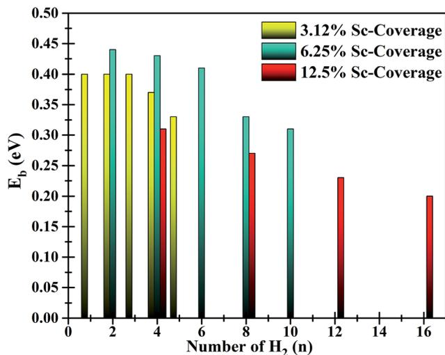
Fig. 6 Adsorption energies of H<sub>2</sub> on functionalized BC<sub>3</sub> sheets for three different values of Sc-coverage.
