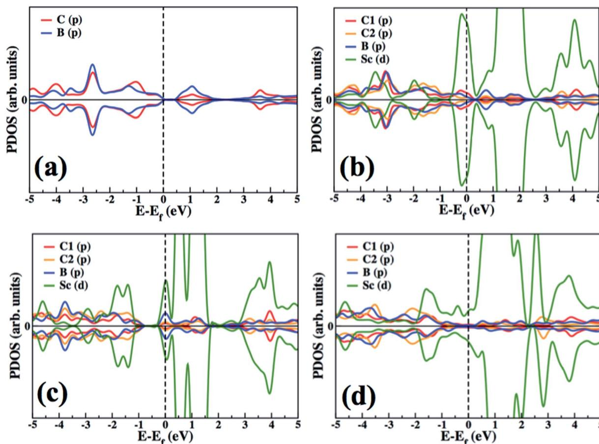
Fig. 4 Partial electronic density of state plots for (a) pure BC<sub>3</sub>, (b) BC<sub>3</sub> with 1 Sc atom [3.12% Sc-coverage], (c) BC<sub>3</sub> with 2 Sc [6.25% Sc-coverage] and (d) BC<sub>3</sub> with 4 Sc [12.5% Sc-coverage]. The dashed line indicates the Fermi level.
