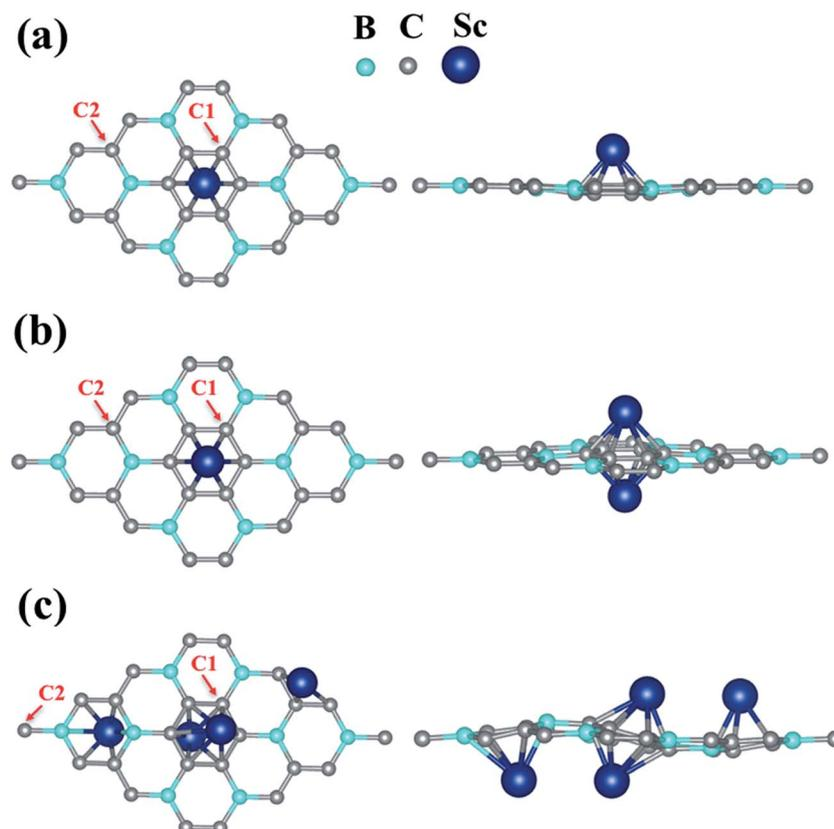
Fig. 2 Top (left) and side (right) views of  $\text{BC}_3$  sheet functionalized with (a) 1 Sc [3.12% Sc-coverage], (b) 2 Sc [6.25% Sc-coverage] and (c) 4 Sc [12.5% Sc-coverage]. C1 and C2 indicate the carbon atoms that were chosen for the plotting of density of states.
