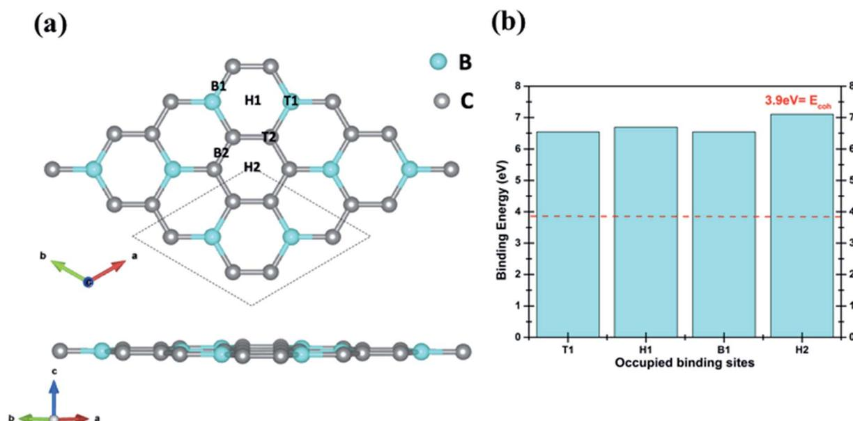
Fig. 1 (a) Top and side view of BC<sub>3</sub> sheet; the primitive cell is marked with dotted lines. High symmetry sites available for adatom occupation are indicated as T1, T2, H1, H2, B1 and B2. (b) Binding energy for occupied binding sites.
