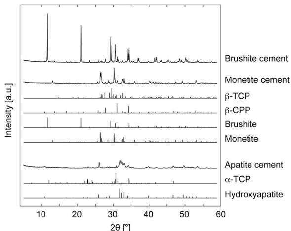
Fig. 8. XRD patterns of set brushite, monetite and apatite cements (one representative pattern out of six for each type of cement is shown) together with reference patterns for identified phases.
