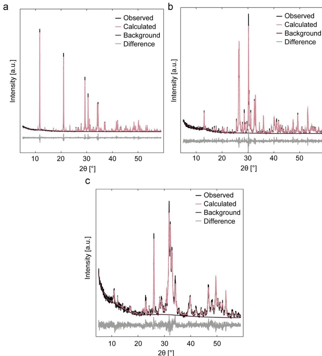
Fig. 9. Representative XRD patterns showing the accuracy of the refinement for a) brushite b) monetite and c) apatite cements.
