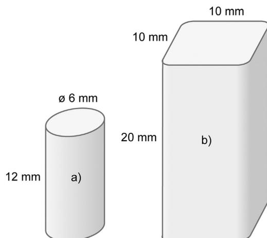
Fig. 1. Specimen geometries used in this study: a) cylindrical specimen and b) rectangular parallelepiped specimen.
