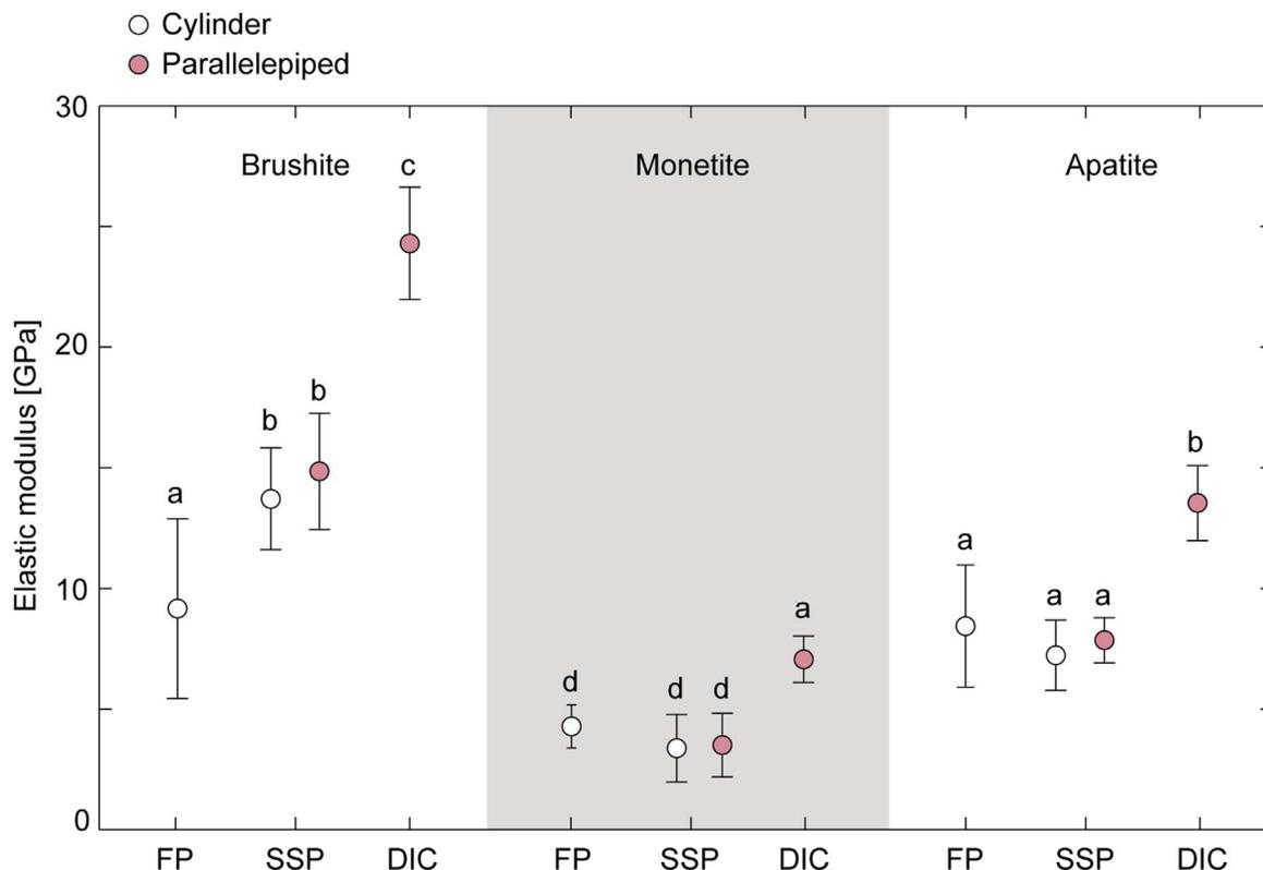
Fig. 5. Elastic modulus of brushite, monetite and apatite cements obtained from FP and SSP, as well as from the DIC-system. Error bar shows one standard deviation. Groups with the same letter are not significantly different.
