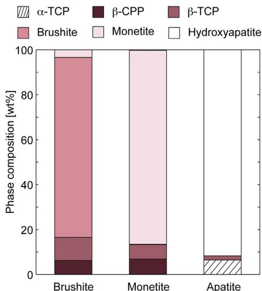
Fig. 7. Phase composition of the three types of cements. Repeatability was equal to or better than 2 wt% for (N = 6 per group).
