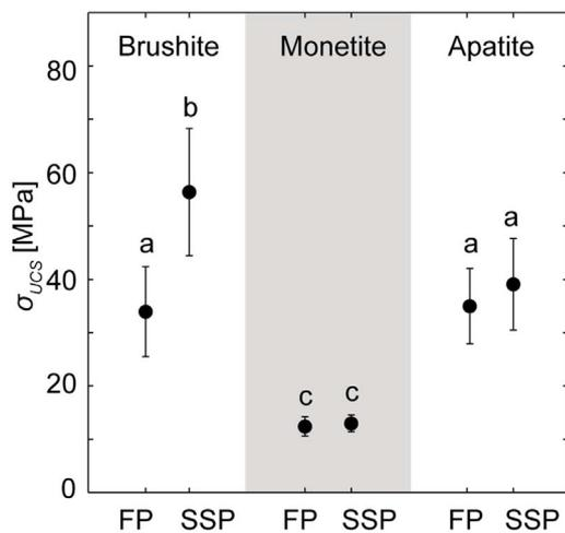
Fig. 3. Mean values of  $\sigma_{UCS}$  for the three types of cements determined from compression testing of cylinders with both FP and SSP (sample size  $N \geq 30$  for all groups). Error bar shows one standard deviation. Groups with the same letter are not significantly different.
