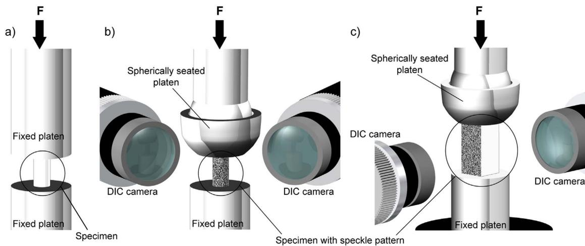
Fig. 2. Schematic of experimental set-up for monotonic compression testing with a) fixed platens (FP), b) spherically seated platens (SSP) and the digital image correlation (DIC) system for 3D measurement and, c) DIC system set-up for 2D measurement.
