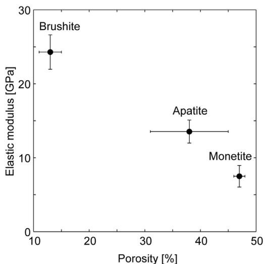
Fig. 6. Elastic modulus (from DIC) as a function of cement type and porosity.
