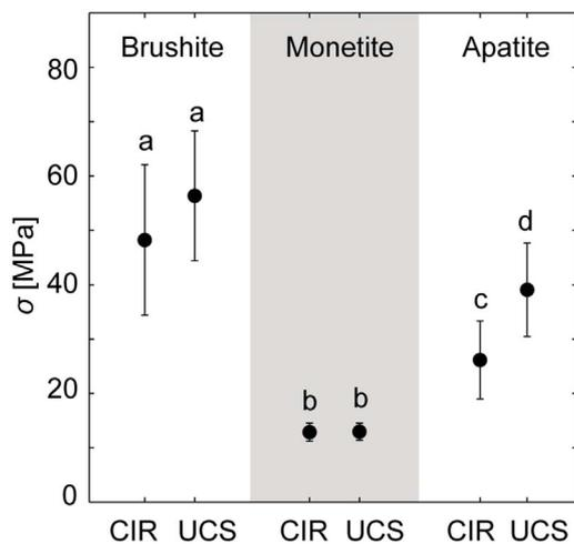
Fig. 4. Mean values of  $\sigma_{CIR}$  and  $\sigma_{UCS}$  for the three types of cements determined from compression testing of cylinders with SSP (sample size  $N = 30$  for all groups). Error bar shows one standard deviation. Groups with the same letter are not significantly different.
