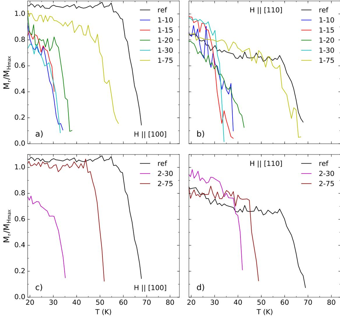
**Figure 3.5:** a) Ratio between remanent magnetisation and maximum field magnetisation  $M_r/M_{Hmax}$  vs. temperature  $T$  with field  $H \parallel [100]$  for superlattices, b)  $M_r/M_{Hmax}$  vs.  $T$  with  $H \parallel [110]$  for superlattices, c)  $M_r/M_{Hmax}$  vs.  $T$  with  $H \parallel [100]$  for multilayers, and d)  $M_r/M_{Hmax}$  vs.  $T$  with  $H \parallel [110]$  for multilayers.
