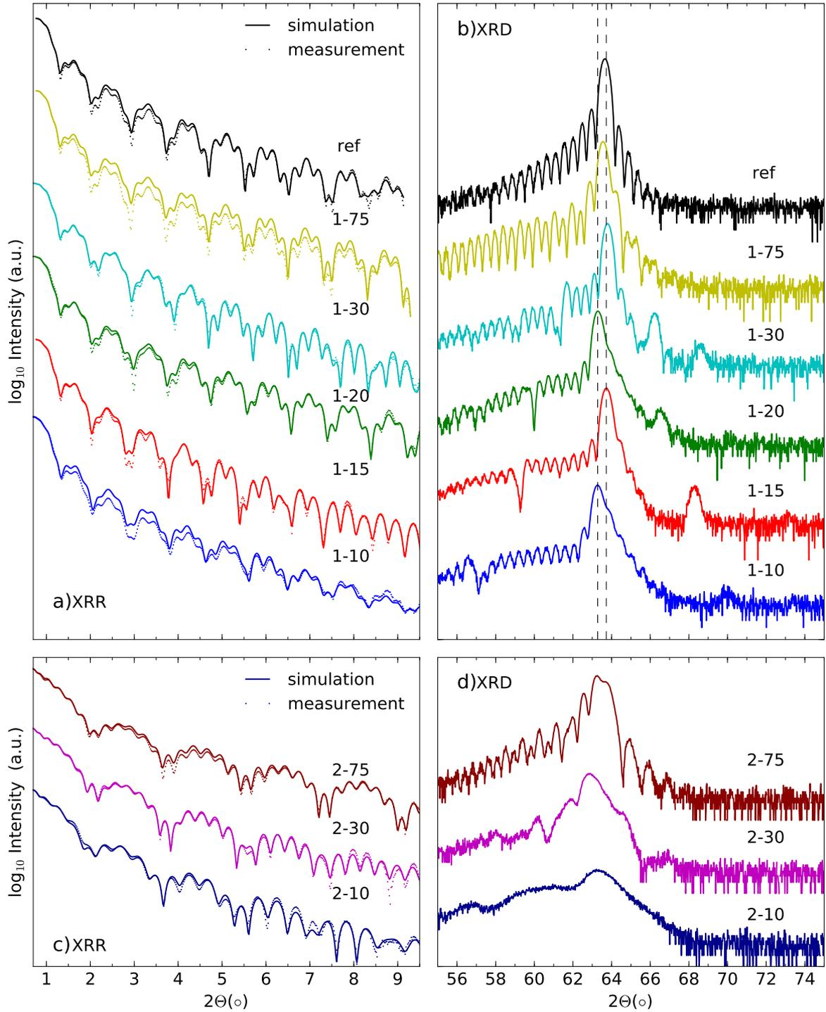
**Figure 3.1:** a) Measured and simulated XRR patterns of the superlattices, b) measured XRD patterns around the (002) peak of the superlattices (the dashed drop-lines are used to indicate that the peak positions of most samples group around two values, corresponding to different strain states of the lattices), c) measured and simulated XRR patterns of the multilayers, and d) measured XRD patterns around the (002) peak of the multilayers.
