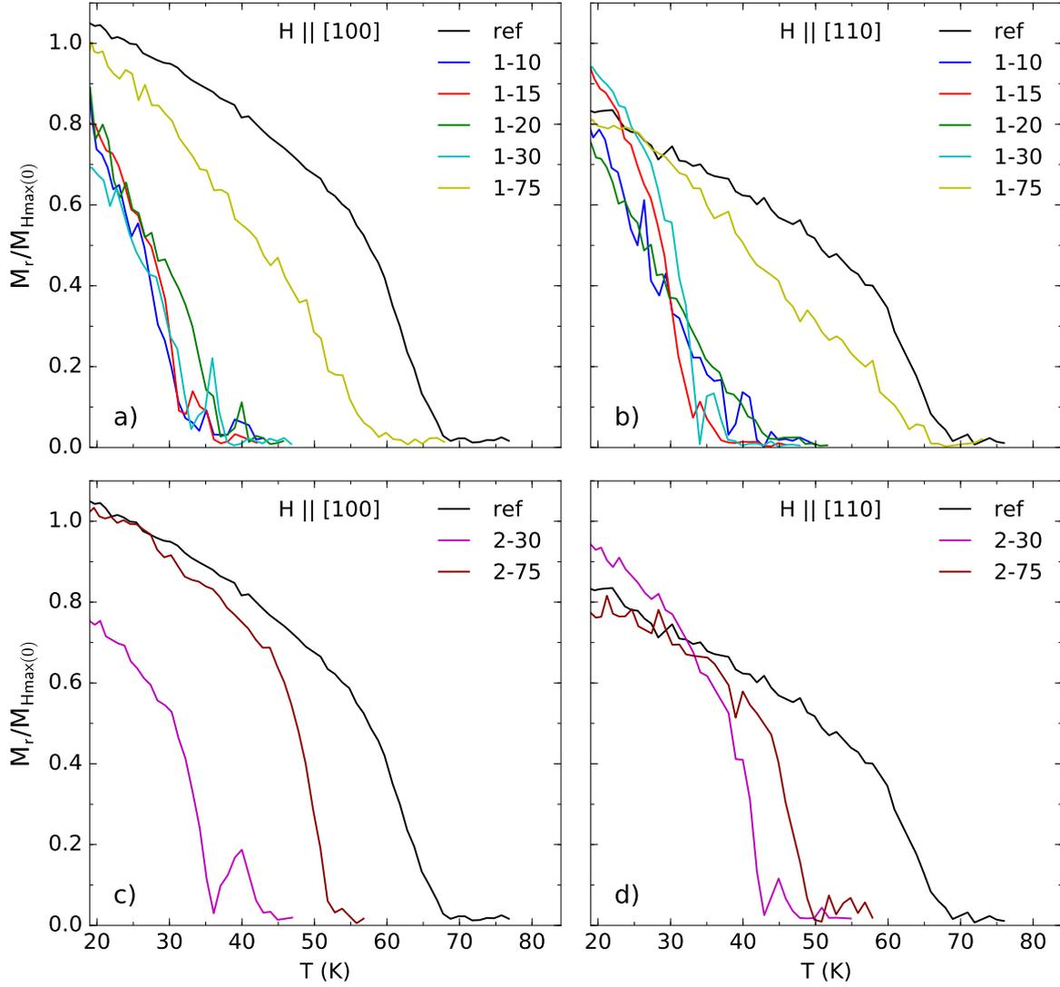
**Figure 3.3:** a) Normalised remanent magnetisation  $M_r/M_{H_{\max}(0)}$  vs. temperature  $T$  with field  $H \parallel [100]$  for superlattices, b)  $M_r/M_{H_{\max}(0)}$  vs.  $T$  with  $H \parallel [110]$  for superlattices, c)  $M_r/M_{H_{\max}(0)}$  vs.  $T$  with  $H \parallel [100]$  for multilayers, and d)  $M_r/M_{H_{\max}(0)}$  vs.  $T$  with  $H \parallel [110]$  for multilayers.
