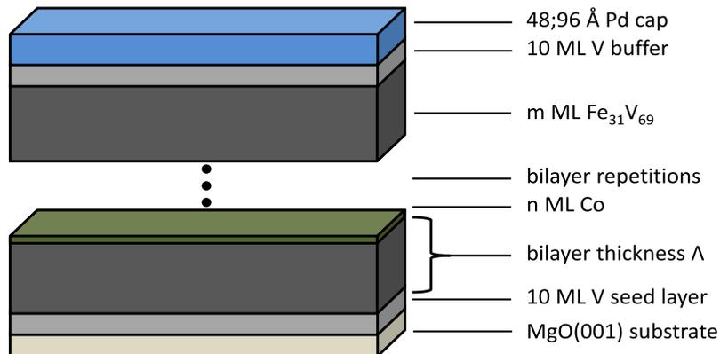
**Figure 2.1:** A schematic representation of the samples. The dashed section represents the repetition of Co/Fe-V bilayers.
