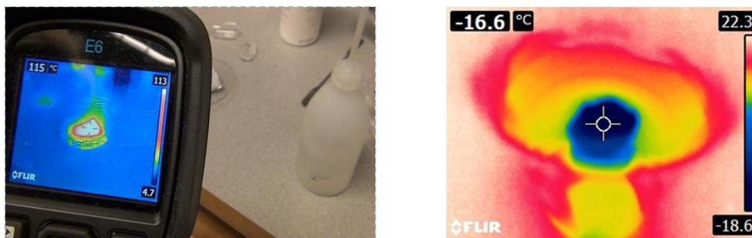
Figure 1. Students use an IR camera to study chemical reactions (left); an IR-camera image of temperature decrease after table salt has been put on an ice cube (right).
