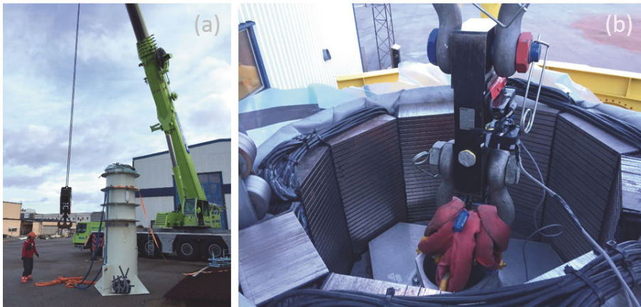
Figure 4.5. (a) The ferrite generator in front of the crane used in the experiment. The generator hull was mounted on a concrete foundation during the experiment. (b) The force sensor was attached between the translator and the crane. The translator is standing on the lower enstop spring in this figure.
