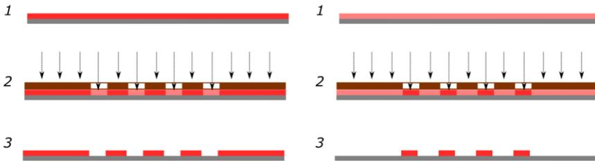
Figure 4 The steps of photolithography. (Left) positive photoresists, (Right) negative photoresists. The process includes (1) formation of a thin film of photoresist on top of the substrate, (2) exposure to light through a photomask and (3) development, removing the exposed part of the positive photoresist, or the non-exposed part of a negative photoresist.
