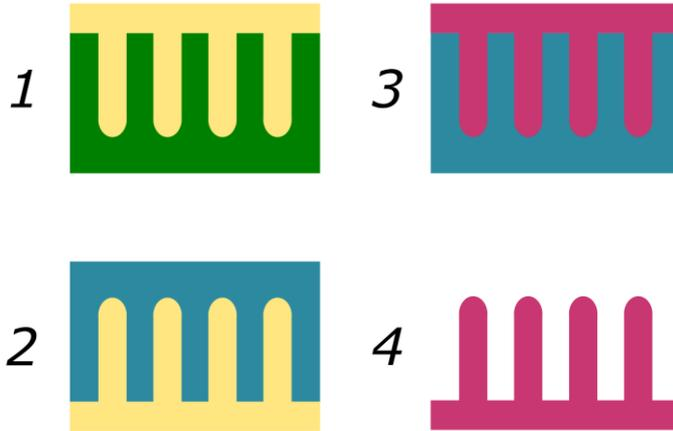
Figure 1 Casting of collagen using PDMS and an alginate sacrificial mold. The fabrication process involves (1) casting of PDMS (yellow) in a plastic mold (green), (2) casting of a sacrificial alginate mold (blue) using the PDMS mold. The collagen (red) is then cast in the alginate mold (3) and as the alginate mold is dissolved leaving only the collagen structure (4).
