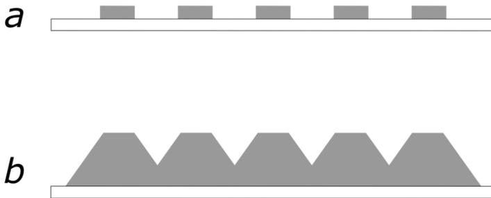
*Figure 7 Photolithography result when using (a) thin polymer films and (b) thick polymer films.*
