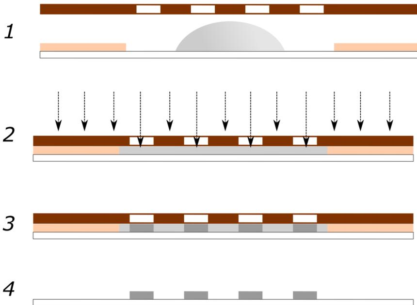
*Figure 6 The steps of photolithography on HA-acrylamide. The process includes (1) formation of a thin film of photoresist between the substrate and the photomask with spacers defining the distance and thus the film thickness, (2) exposure to light through a photomask and (3) development in water or PBS, washing off any non-crosslinked part of the hydrogel solution.*
