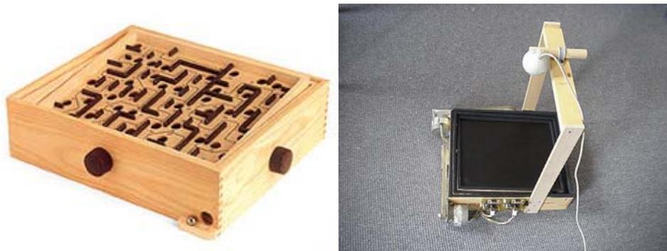
*Figure 1 A Brio labyrinth, and a modified version with a camera and motors added*
