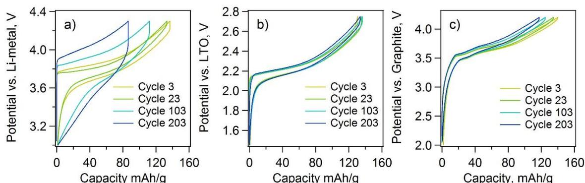
Figure 1. Potential profiles of NMC electrodes cycled versus different negative electrodes. a) NMC vs. Li-metal. b) NMC vs. LTO. c) NMC vs. graphite.
