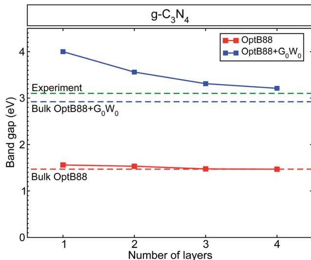
Fig. 1 The calculated band gap for graphitic-like  $C_3N_4$  as a function of the number of layers. We have included as a reference the calculated band gap for bulk g-h-triazine with OptB88 (red dashed line), OptB88+ $G_0W_0$  (blue dashed line), and the experimental value<sup>40</sup> (green dashed line).
