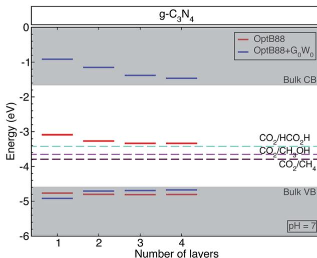
Fig. 2 The calculated band edges for graphitic-like  $C_3N_4$  as a function of the number of layers. The gray shaded areas show the valence and conduction bands for bulk g-h-triazine calculated with OptB88+ $G_0W_0$ . We have also added, for comparison, the measured reduction reactions producing methane  $CH_4$ , methanol  $CH_3OH$ , and formic acid  $HCO_2H$  at pH = 7.
