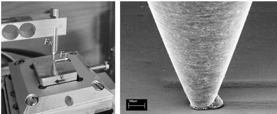
*Fig. 5. To the left; the in situ test equipment. To the right; aluminium tip in sliding contact with a tool steel flat.*
