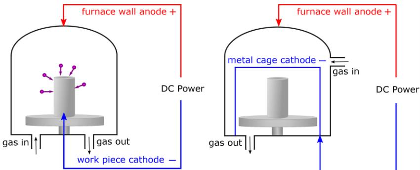
Fig. 2. Left: Regular plasma nitriding; Right: Active-screen plasma nitriding
