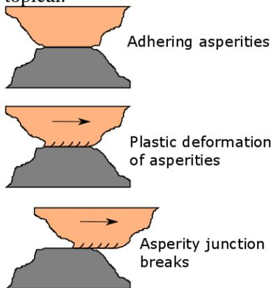
*Fig. 4. A schematic of the adhesion model.*
