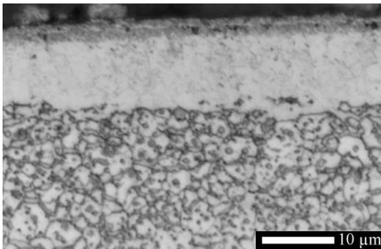
*Fig. 1. A polished cross section of a nitrocarburized Orvar steel sample depicted with a light-optic microscope. The light grey area is the compound layer. It appears that the area closest to the surface is porous.*
