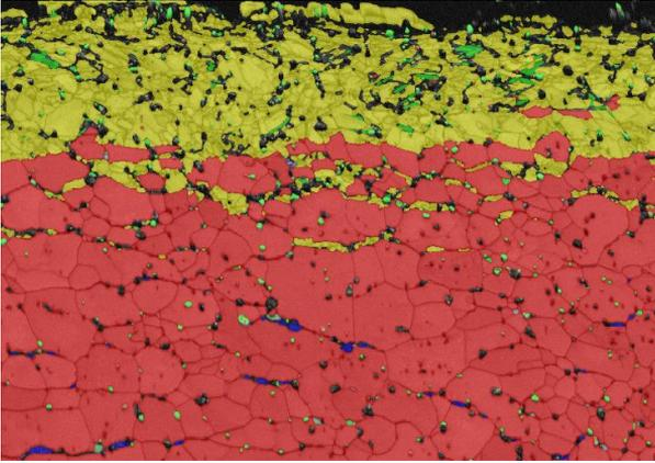
*Fig. 3. A crystal structure map of a polished cross section of a nitrocarburized Orvar steel sample. The  $\epsilon$ -phase in the compound layer is shown in yellow and the  $\gamma'$ -phase is shown in green. The blue areas represent cementite and the red area the steel substrate.*
