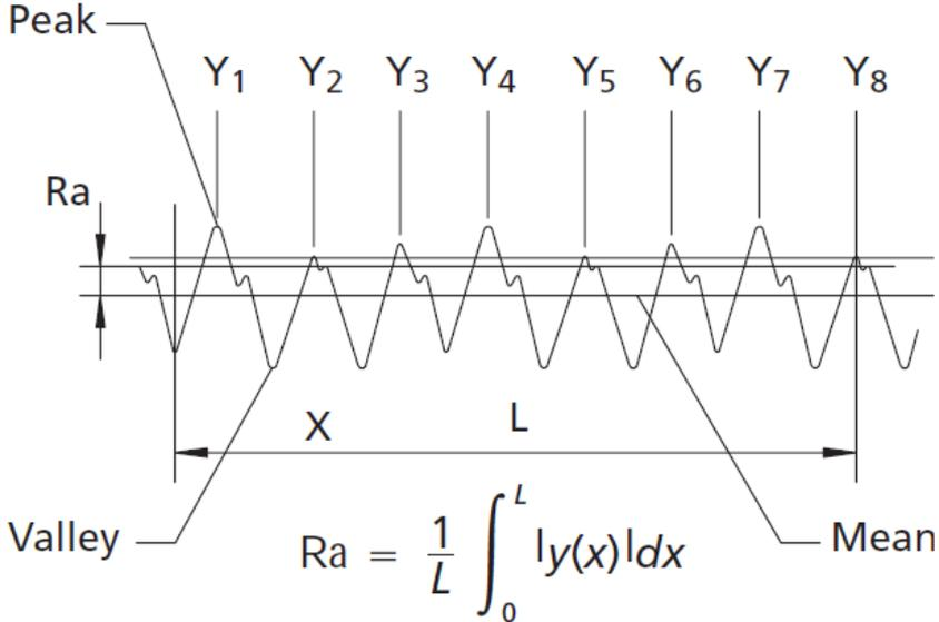
*Fig. 6. The arithmetic average roughness value, Ra.*
