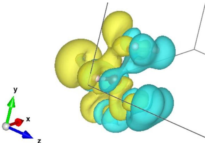
Figure 5: *This figure is a visualisation, generated in VESTA [10], of the change in electron density between the state with no external electric field and the state with a field of  $0.090 \text{ V/\AA}$  in the  $\hat{z}$ -direction for alanine. The electrons have moved from the blue areas to the yellow areas. The iso-surface level is here  $7.9 \times 10^{-5} e/a_0^3$ , where  $a_0$  is the Bohr radius.*
