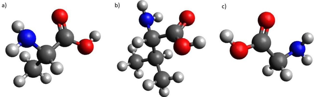
Figure 2: The three amino-acids of the project are here depicted by the use of Avogadro. The red spheres represent oxygen, the dark grey represent carbon, the lighter grey represent hydrogen and the blue represent nitrogen. The chemical formulas are respectively  $C_3H_7NO_2$ ,  $C_5H_{11}NO_2$  and  $C_2H_5NO_2$  for alanine (a), valine (b) and glycine (c).
