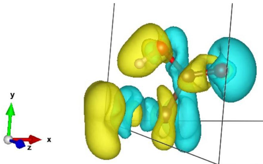
Figure 9: *This figure is a visualisation, generated in VESTA, of the change in electron density between the state with no external electric field and the state with a field of  $0.068 \text{ V/\AA}$  in the  $\hat{x}$ -direction for glycine. The electrons have moved from the blue areas to the yellow areas. The iso-surface level is here  $6.0 \times 10^{-5} e/a_0^3$ , where  $a_0$  is the Bohr radius.*
