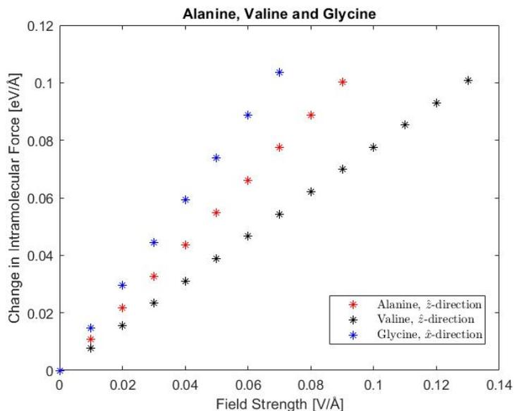
Figure 3: The absolute value of the largest change in the intramolecular forces of alanine, valine and glycine are here plotted against the corresponding field strengths. The three sets of data corresponds to the weakest field strengths required for a change of  $0.1 \text{ eV}/\text{\AA}$  in the intramolecular forces for each amino-acid respectively.
