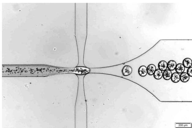
**Figure 1:** Microfluidic production of HA-am droplets with 10  $\mu\text{m}$  sized polystyrene beads with flows of 5  $\mu\text{l min}^{-1}$  on the aqueous phase and 15  $\mu\text{l min}^{-1}$  of the fluorinated oil phase per each of the 2 inlets. Scale bars correspond to 200  $\mu\text{m}$ .
