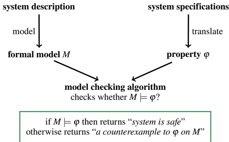
Figure 1.2. Basic form of model checking.
