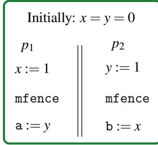
Figure 1.9. Dekker’s mutual exclusion algorithm with fences inserted for correct operation under TSO.
