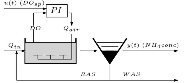
Fig. 1. Simulation model.  $Q_{in}$ -inflow,  $u(t)$ -input signal ( $DO_{sp}$ -DO set point),  $PI$ -proportional integral DO controller,  $Q_{air}$ -airflow rate,  $y(t)$ -output signal ( $NH_4 conc$ -ammonium concentration)  $RAS$ -return activated sludge,  $WAS$ -waste activated sludge.
