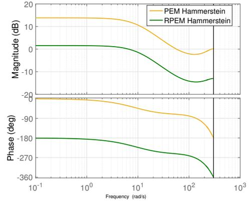
Fig. 7. Bode plot of the linear part obtained with PEM and RPEM Hammerstein models.
