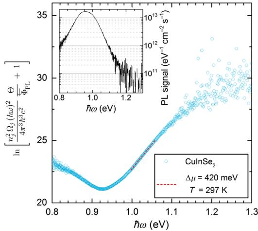
FIG. 2. Determination of  $\Delta\mu$  and  $k_B T$  from a linear fit in the high-energy range of the PL signal for a  $\text{CuInSe}_2$  thin film deposited on a soda-lime glass substrate. The optical factor  $\Theta$  is determined from transmittance and reflectance measurements on the thin film plus substrate and on the bare substrate. (Inset) The corresponding PL spectrum for an emission in the  $2\pi$  sr in front of the sample.
