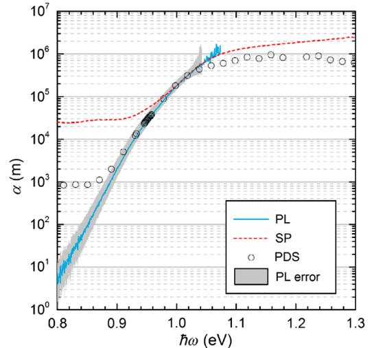
FIG. 3. Comparison of the absorption coefficient of a  $\text{CuInSe}_2$  thin film deposited on soda-lime glass substrate measured by various methods (PL, photoluminescence; SP, spectrophotometry; PDS, photothermal deflection spectroscopy).
