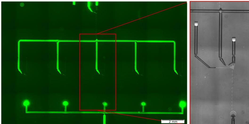
Left: Microfluidic chip with five units in parallel and one coupled in series concentrating 1  $\mu\text{m}$  fluorescent particles. The recovery was 97% at a concentration factor of 35 with at a throughput of 200  $\mu\text{l}/\text{min}$  and a pressure drop of 60 bar. Right: Single unit. It consists of a shallow horse shoe channel with deep and wide interconnects.
