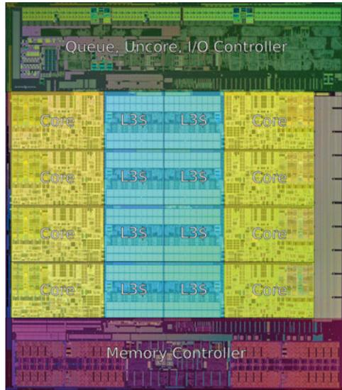
**Figure 21:** Thermal imaging of the silicon die of an octa-core Intel Haswell processor. The total area of the distributed L3 Cache, highlighted in light blue, is comparable in size with the total area of the eight cores, highlighted in light yellow. Note that the area in yellow, attributed to cores, includes at least a D-Cache, an I-Cache and an L2-Cache. (Image source: WikiChip November 01, 2018; use permitted under the Creative Commons Attribution License CC BY 3.0.)
