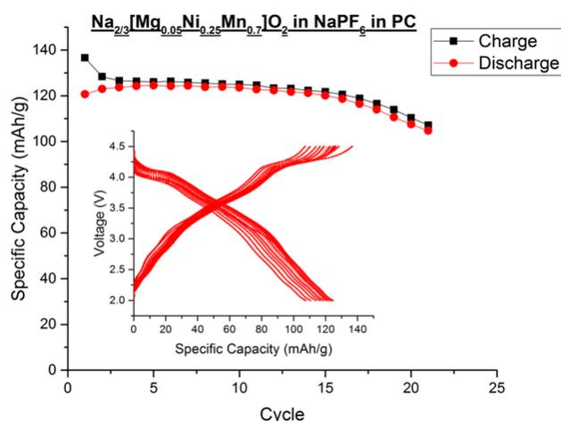
Fig. 1. Galvanostatic charge/discharge curve of  $\text{Na}_{0.67}\text{Ni}_{0.25}\text{Mg}_{0.05}\text{Mn}_{0.7}\text{O}_2$
