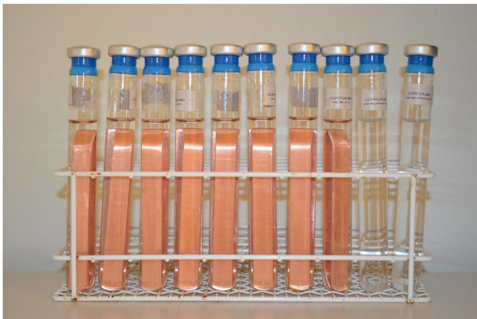
Fig. 1. Pairs of copper pieces immersed in pure water, contained in butyl rubber sealed borosilicate glass tubes. The  $6\text{ cm}^3$  gas phase at the top is sampled and analysed at regular intervals. Two tubes contain only water and gas. The image was taken after 27 months of exposure to pure, oxygen-free water at  $70^\circ\text{C}$ .
