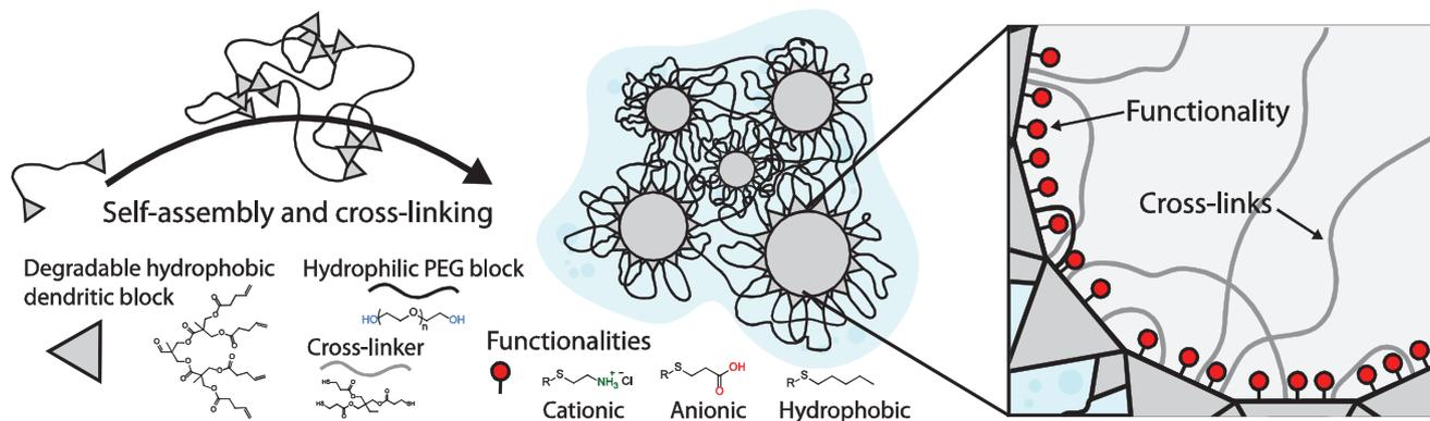
**Figure 1.** Purposed structure of dendritic nanogels (DNGs) constructed from amphiphilic linear dendritic hybrids between poly(ethylene glycol) (PEG) and 2,2-bis(hydroxymethyl)propionic acid (bis-MPA). Created DNGs can further be functionalized to display both anionic, cationic, and hydrophobic interior while maintaining size and hydrophilic PEG exterior. This enables DNGs to be tailor-made to load and deliver different cargos.
