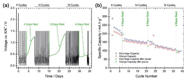
Fig. 4 (a) Voltage profile of a pause test at  $25 \text{ mA g}^{-1}$  using BMG as the working electrode. Potential limitations of  $0.01 \text{ V}$  and  $1.5 \text{ V}$  vs.  $\text{K/K}^+$  were used with the following cycling regime: 6 cycles, rest 4 days, 14 cycles, rest 8 days, 16 cycles, rest 4 days, continued cycling. (b) Specific capacity for galvanostatic discharge/charge cycles during the pause test.
