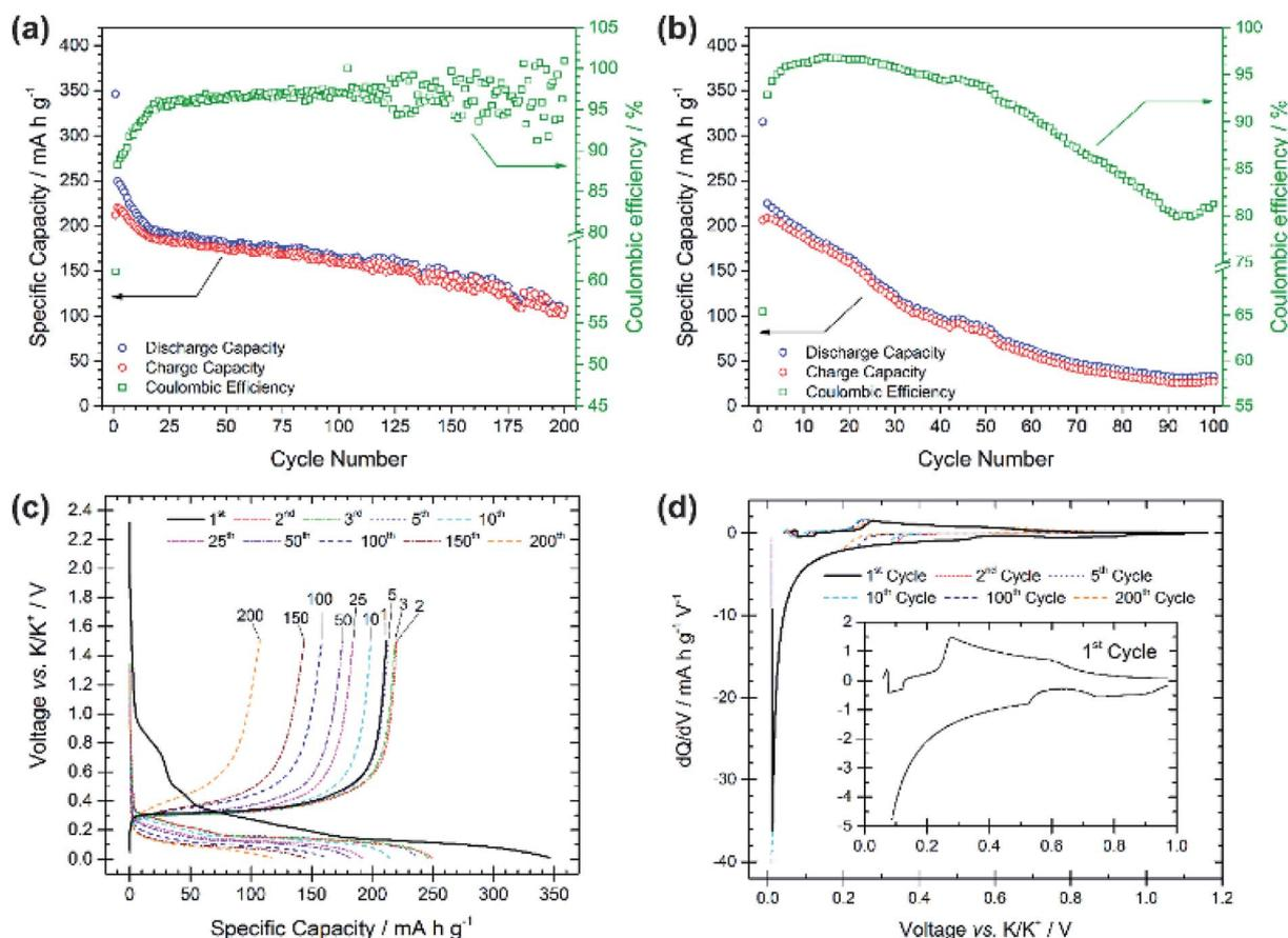
Fig. 3 Specific capacity vs. cycle number for the ball-milled graphite (BMG) electrode galvanostatically cycled at (a)  $25 \text{ mA g}^{-1}$  and (b)  $250 \text{ mA g}^{-1}$  with potential limitations of 0.01 V and 1.5 V vs. K/K<sup>+</sup>. (c) Voltage profiles vs. specific capacity for selected cycle numbers from the test at  $25 \text{ mA g}^{-1}$ . (d)  $dQ/dV$  plots for cycles 1, 2, 5, 10, 100, and 200 from the test at  $25 \text{ mA g}^{-1}$ .
