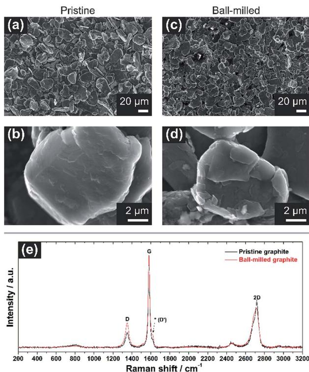
**Fig. 1** (a and b) SEM images of the pristine graphite (PG) electrode at low (1000 $\times$ ) and high (20 000 $\times$ ) magnification. (c and d) SEM micrographs of ball-milled graphite (BMG) electrode at low and high magnification. (e) Normalized Raman spectra of pristine (black) and ball-milled graphite (red). Note the increase of the relative intensity of the 'D' band in (e) after ball-milling, as well as a more prominent signal at  $\sim 1620\text{ cm}^{-1}$  (see asterisk).
