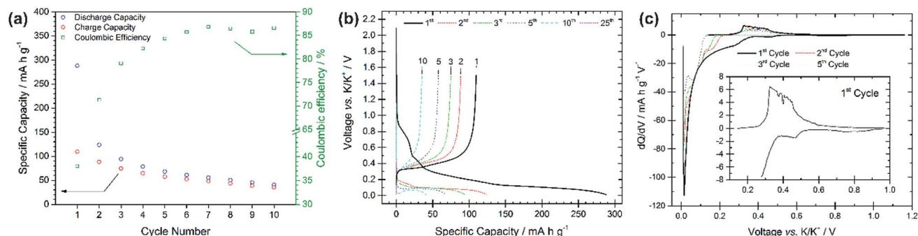
**Fig. 2** (a) Specific capacity vs. cycle number for the pristine graphite electrode galvanostatically cycled at  $25\text{ mA g}^{-1}$  with potential limitations of 0.01 V and 1.5 V vs. K/K<sup>+</sup>. (b) Voltage profiles vs. specific capacity for selected cycle numbers from the same test. (c)  $dQ/dV$  plots for cycles 1, 2, 3 and 5 for the same test.
