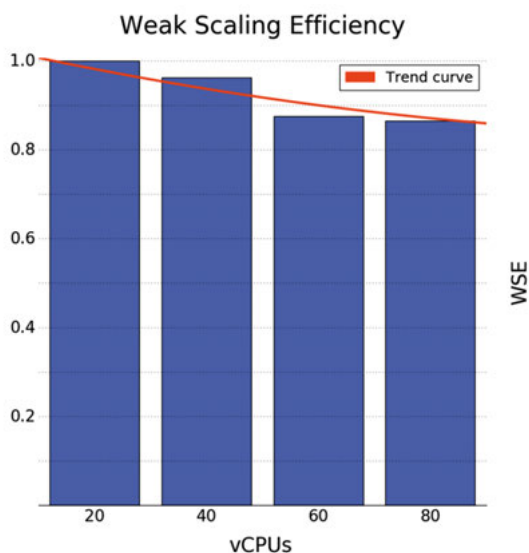
Figure 4.4. Weak scaling efficiency for the Spark-based virtual screening implementation. The Weak Scaling Efficiency (WSE) is a performance metric that shows how well a system scales when increasing both the problem size and the processing units – virtual Central Processing Units (vCPUs) in this case – such that the amount of work per processing unit stays constant. This plot shows the WSEs for a virtual screening analysis over the SureChEMBL dataset [119] retrieved in ready-to-dock format from the ZINC database [120]. More information about the experimental settings can be found in Paper II.
