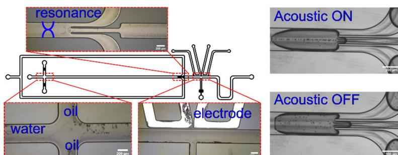
**Figure 1:** The design of the chip for droplet generation and washing. Droplets with high background noise are generated via flow focusing at the channel junction. A half wavelength acoustic standing wave field is generated in the channel which focuses the beads along the central line of the droplets. The droplets are split into three daughter droplets at the trifurcation. After droplet splitting, the droplets are refilled with fresh fluid to the original volume by the pico-injector.
