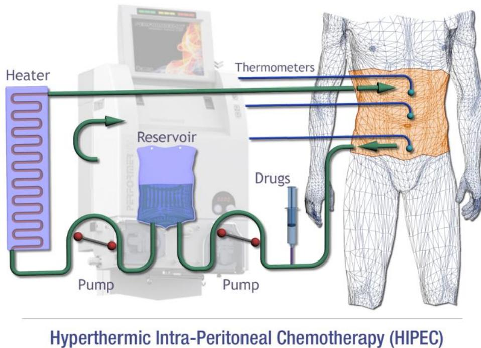
Figure 2: A schematic drawing of a HIPEC setup.
