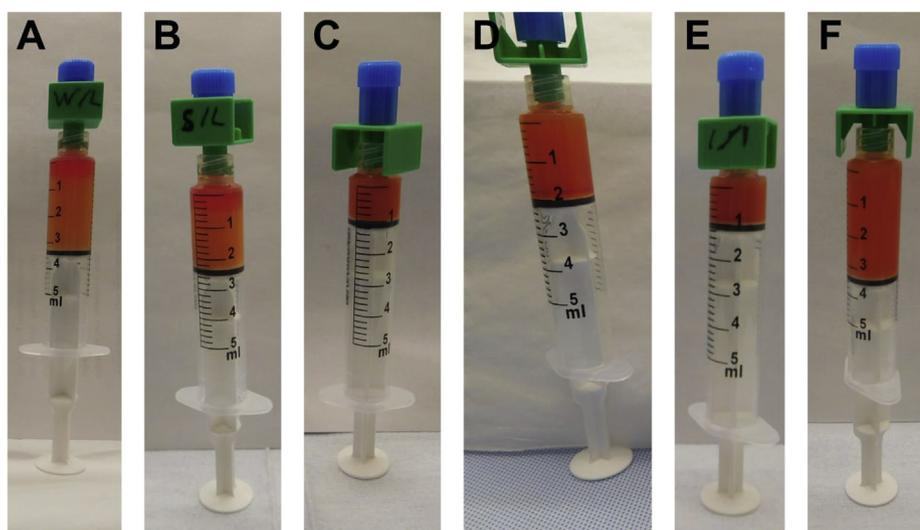
Fig. 4. Visual inspection of the stability of the emulsions at the 1 hr time point. Separated emulsions: A) water and Lipiodol® (W/L) aqueous-to-lipid phase ratio of 1:4, B) saline 0.9% and Lipiodol® (S/L) aqueous-to-lipid phase ratio of 1:4. Maintained emulsions: C) and D) iohexol and Lipiodol® (I/L) aqueous-to-lipid phase ratio of 1:1 and 1:4 respectively, E) and F) mixture (v/v) of iohexol (85%)/water (15%) and Lipiodol® (IW/L) aqueous-to-lipid phase ratio of 1:1 and 1:4 respectively.
