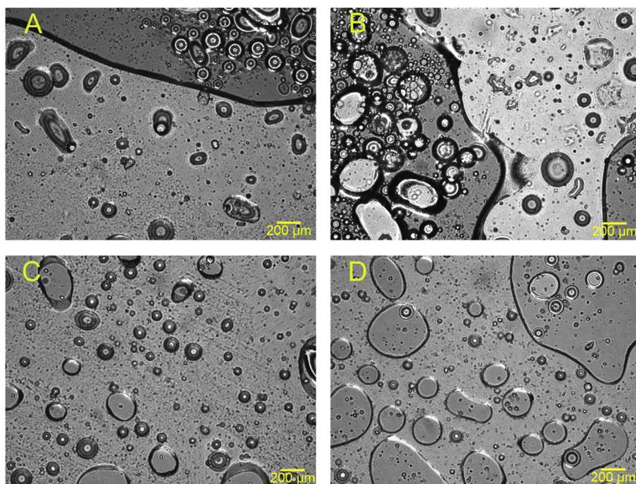
Fig. 5. Microscope images of emulsions with aqueous phase composition of water (W/L) and saline 0.9% (S/L) at 15 min time point. A) Emulsion W/L aqueous-to-lipid phase ratio of 1:1, B) Emulsion S/L aqueous-to-lipid phase ratio of 1:1, C) Emulsion W/L aqueous-to-lipid phase ratio of 1:4 and D) Emulsion S/L aqueous-to-lipid phase ratio of 1:4. All images are at 20 × magnification.
