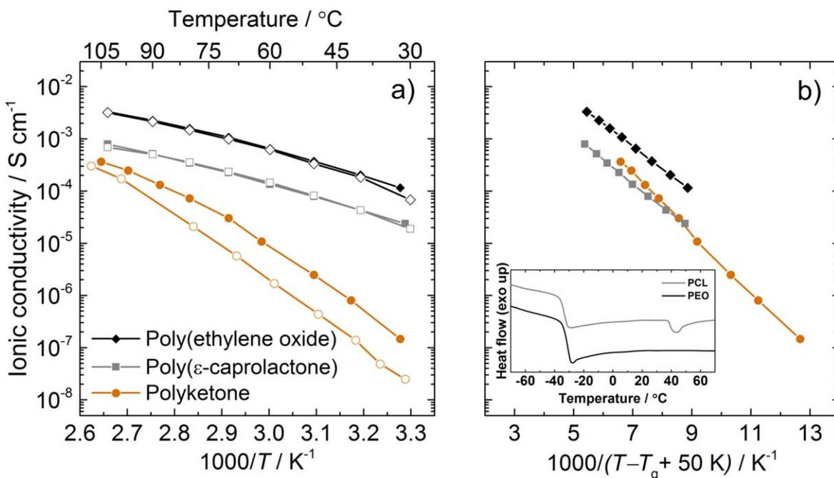
**Figure 6.** Total ionic conductivity of electrolytes based on the polyketone, PEO and PCL, respectively (all with an O:Li<sup>+</sup> ratio of 10) plotted against (a)  $1000/T$  and (b) the shifted temperature scale  $1000/(T - T_g + 50 \text{ K})$ . The inset in (b) shows DSC data for the PCL and PEO electrolytes. Open markers indicate measurements during heating and filled markers indicate measurements during cooling.
