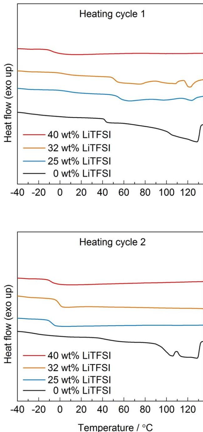
**Figure 3.** DSC scans for the poly(3,3-dimethylpentane-2,4-dione) without LiTFSI and with 25, 32 or 40 wt% LiTFSI for heating cycle 1 and 2.
