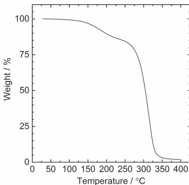
**Figure 2.** Thermogravimetric analysis of the polymer without salt from room temperature up to 400 °C.
