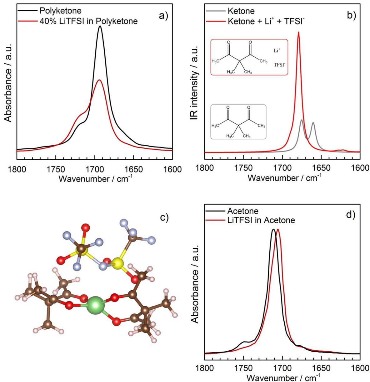
**Figure 4.** (a) Experimental FT-IR spectra of the polyketone with and without LiTFSI; (b) calculated FT-IR spectra of a diketone mimic by itself and in the presence of a Li<sup>+</sup> and a TFSI<sup>-</sup>; (c) illustration of coordination between Li<sup>+</sup> (green) and four oxygens (red) of two ketone molecules; and (d) experimental FT-IR spectra of acetone with or without LiTFSI.
