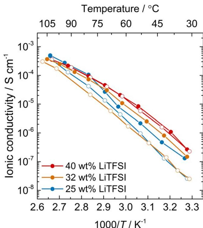
**Figure 5.** Total ionic conductivity data for the polyketone samples containing 25, 32 or 40 wt% LiTFSI. Open markers indicate measurements during heating and filled markers indicate measurements during cooling.
