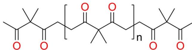
**Figure 1.** Chemical structure of the poly(3,3-dimethylpentane-2,4-dione) polyketone used in this work.
