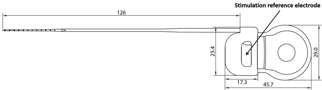
**Figure 2.** Electrode sketch, stimulation reference electrode (arrow) on the implant housing (MED-EL<sup>®</sup>, Innsbruck, Austria). Electrode contact 1 is at the tip of the implant array and electrode contact 12 is closest to the implant housing.
