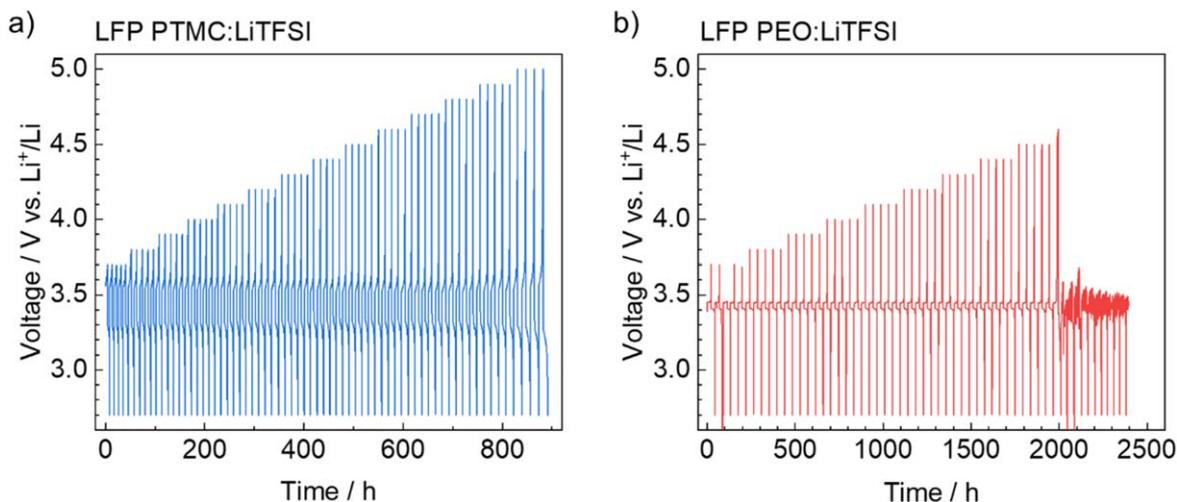
**Figure 5.** Voltage vs time profiles with the CICC method, where the upper cut-off voltage is increased every 5 cycles, for LFP half-cells with (a) PTMC:LiTFSI and (b) PEO:LiTFSI.
