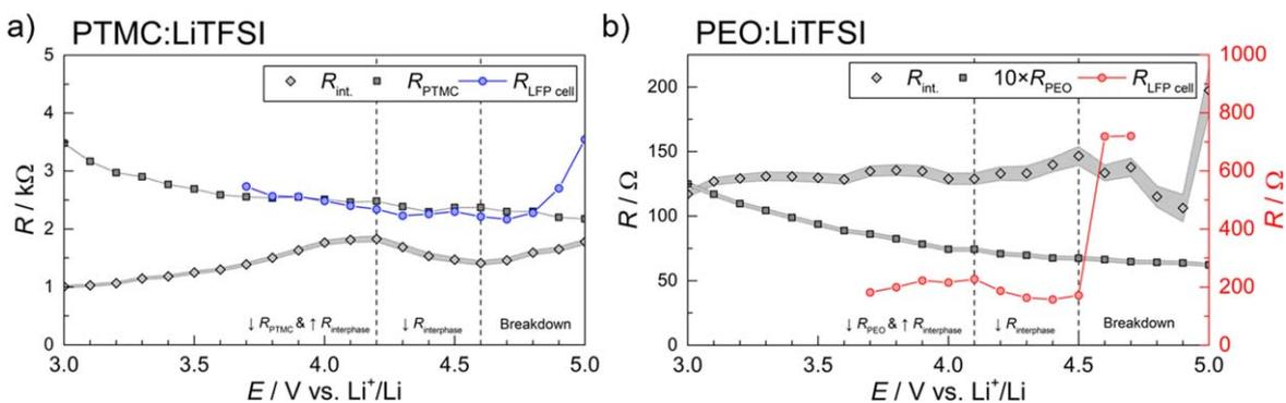
**Figure 7.** The bulk polymer resistance ( $R_{\text{bulk}}$ ) and interfacial resistance ( $R_{\text{int}}$ ) from EIS, and the internal cell resistance from ICI ( $R_{\text{LFP cell}}$ ) for a) PTMC:LiTFSI and b) PEO:LiTFSI at different potential steps.  $R_{\text{PEO}}$  has been multiplied by 10 to improve legibility. The absolute error for  $R_{\text{int}}$ ,  $R_{\text{PTMC}}$ ,  $R_{\text{PEO}}$  and  $R_{\text{tot}}$  is represented by the shaded area.
