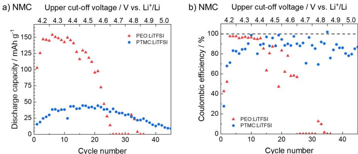
**Figure 8.** Results from CICC experiments for NMC half-cells: a) discharge capacity and b) Coulombic efficiency. The first employed upper cut-off voltage is 4.2 V vs Li<sup>+</sup>/Li and it was thereafter increased by 0.1 V every 5 cycles until 5 V vs Li<sup>+</sup>/Li or until battery failure.
