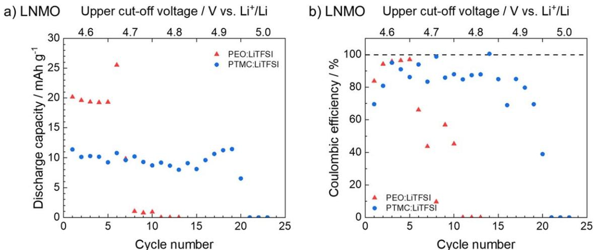
**Figure 9.** Results from CICC experiments for LNMO half-cells: a) discharge capacity and b) Coulombic efficiency. The first upper cut-off voltage employed is 4.6 V vs Li<sup>+</sup>/Li and it was thereafter increased by 0.1 V every 5 cycles until 5 V vs Li<sup>+</sup>/Li or until battery failure.
