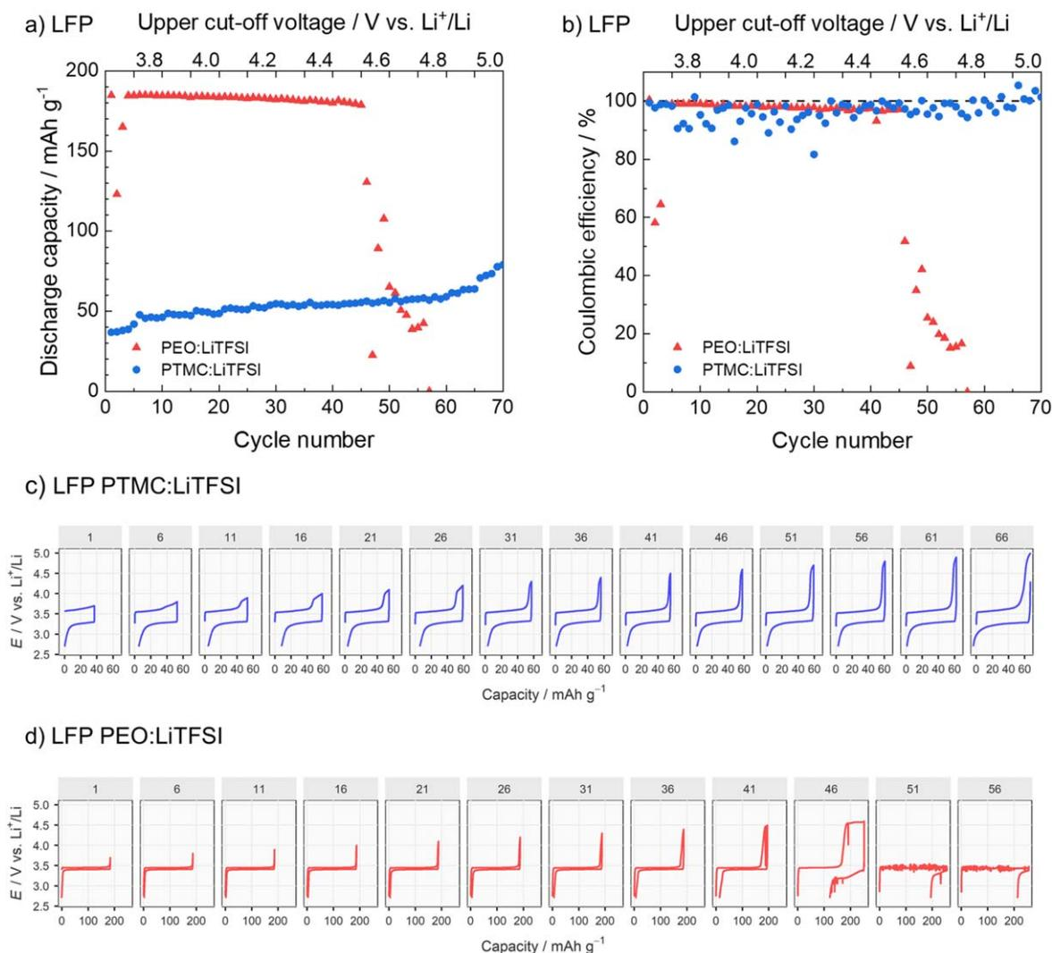
**Figure 6.** Results from the CICC method for LFP half-cells: (a) discharge capacity, (b) coulombic efficiency, (c) and (d) voltage profiles with PTMC:LiTFSI and PEO:LiTFSI, respectively, at different cycles with each cut-off voltage. The first upper cut-off voltage is 3.7 V vs Li<sup>+</sup>/Li and it is increased with 0.1 V every 5 cycles until 5 V vs Li<sup>+</sup>/Li or battery failure.
