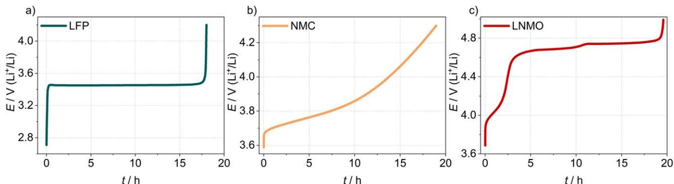
**Figure 3.** Delithiation profile of the 5th cycle of (a) LFP, (b) NMC, and (c) LNMO half-cells at C/20 with liquid electrolyte (LP40) at room temperature.
