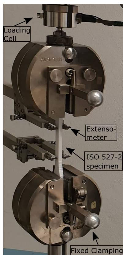
**Figure 4.** Initial state of an ISO 527-2 specimen clamped into a Zwick 1446 testing device with an extensometer (left) and a loading cell (top). One mounting side is fixed (bottom), while displacement is applied vertically through the upper mounting side.
