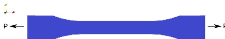
Figure 5. An illustration of the ISO 527-2 CAD model with boundary conditions.
