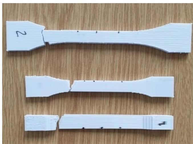
(a) Geometries: ISO-modified, ISO 527-2, ASTM D3039 angle. Failures of Slicing B.
