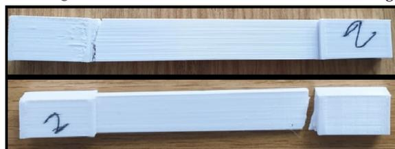
(c) Geometries: ASTM D3039, Top: Slicing B, Down: Slicing A
