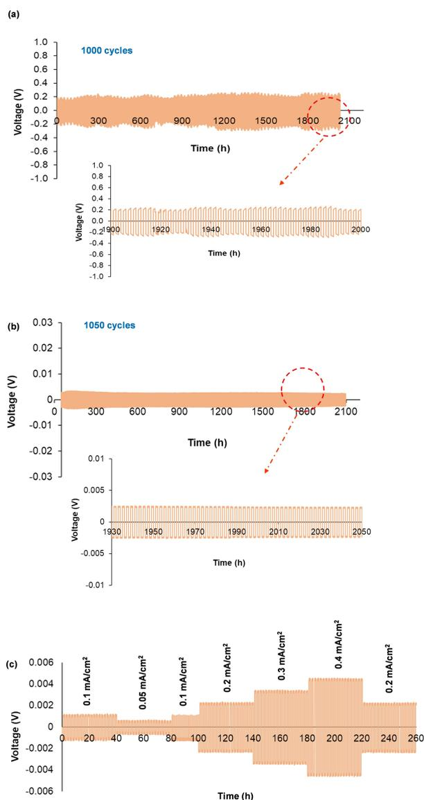
**Figure 5.** Lithium stripping/plating tests for a)  $P(\text{CL}_{80}\text{TMC}_{20})\text{-LiTFSI}_{0.28}$  (no filler), b)  $P(\text{CL}_{80}\text{TMC}_{20})\text{-LiTFSI}_{0.28}\text{-ZrO}_2$  (4 wt.%) at a current density of  $0.2 \text{ mA cm}^{-2}$  and c)  $P(\text{CL}_{80}\text{TMC}_{20})\text{-LiTFSI}_{0.28}\text{-ZrO}_2$  (4 wt.%) at varying current densities ( $0.1\text{--}0.4 \text{ mA cm}^{-2}$ ).
