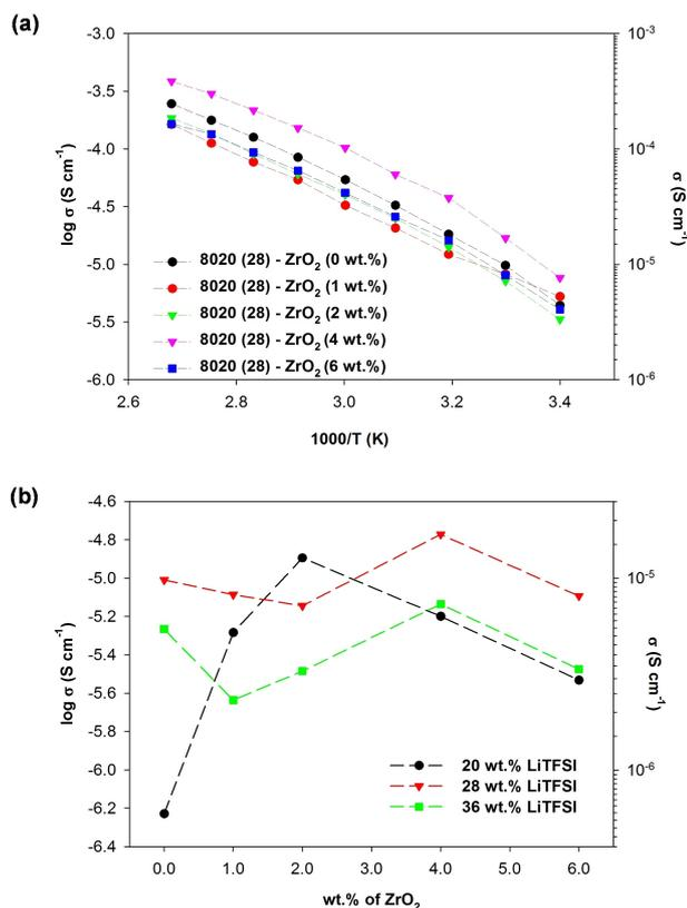
**Figure 4.** Ionic conductivities for a)  $P(\text{CL}_{80}\text{TMC}_{20})\text{-LiTFSI}_{0.28}$  with different wt.% zirconia nanoparticles and b) graph of ionic conductivities at 30 °C. Corresponding plots for 20 wt.% of LiTFSI and 36 wt.% of LiTFSI is shown in Figure S4.
