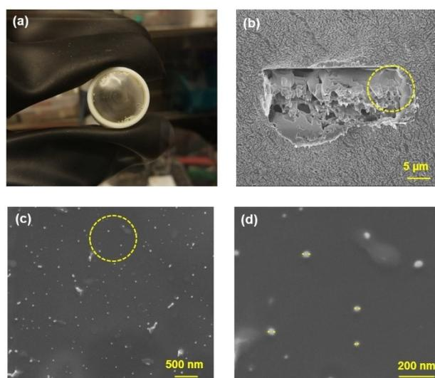
**Figure 1.** Photograph and SEM micrographs of P(CL<sub>80</sub>TMC<sub>20</sub>)–LiTFSI<sub>0.28</sub>–ZrO<sub>2</sub> (4 wt.%) obtained from FIB-SEM: a) NCPE film after the drying process, b) pool-shaped cavity from milling the surface of the film, c) zirconia nanoparticles at the walls of the cavity, circled in (b), and (d) an enlarged image of the SEM micrograph, circled in (c).
