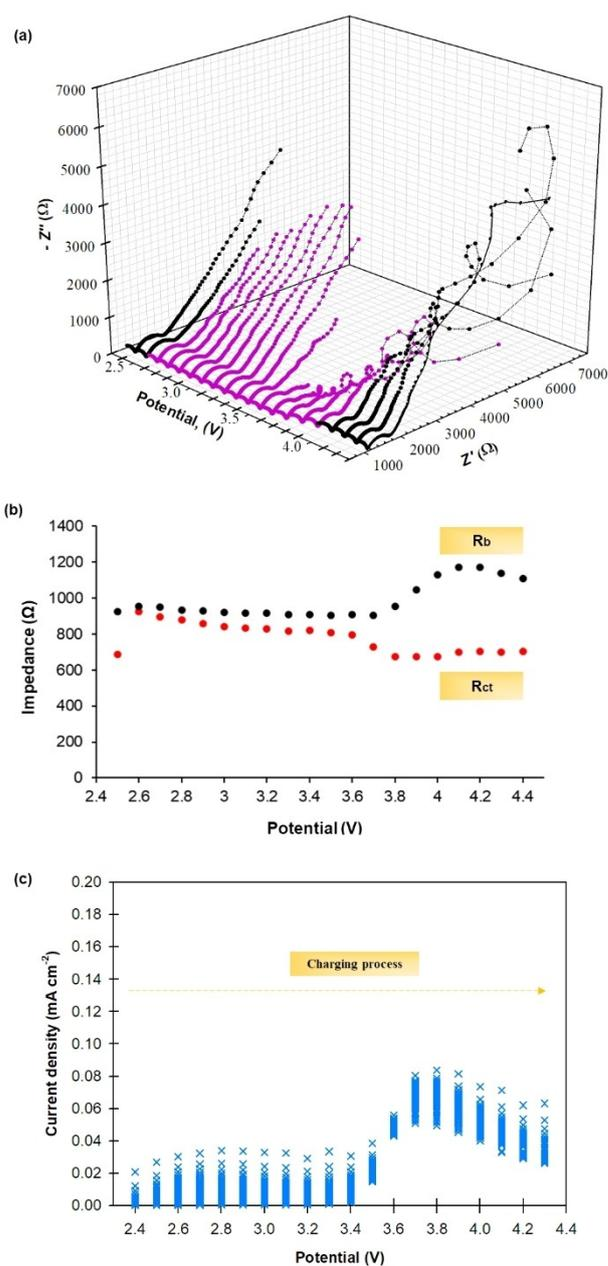
**Figure 7.** a) DEIS profile of a Li/P(CL<sub>80</sub>TMC<sub>20</sub>)–LiTFSI<sub>0.28</sub>–ZrO<sub>2</sub> (4 wt.%) / LFP cell, b) the  $R_{CT}$  and  $R_b$  plotted vs potential (impedance data fitted to a Debye circuit ( $Q1/R1 + Q2/R2$ )) and c) current density vs potential derived from DEIS.
