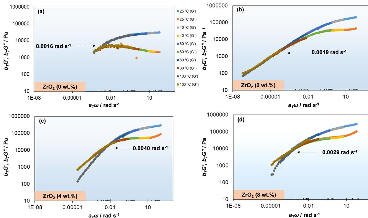
**Figure 3.** Rheological frequency sweep test ( $G'$  and  $G''$  vs frequency) for temperatures 25–100 °C (reference temperature 25 °C) of  $P(\text{CL}_{80}\text{TMC}_{20})\text{--LiTFSI}_{0.28}\text{--ZrO}_2$  at various concentrations of zirconia nanoparticles. Temperature is indicated as different colors. The cross-over frequency of  $G'$  and  $G''$  is indicated for each master curve. The  $a_T\omega$ -shift plots are shown in Figure S3.
