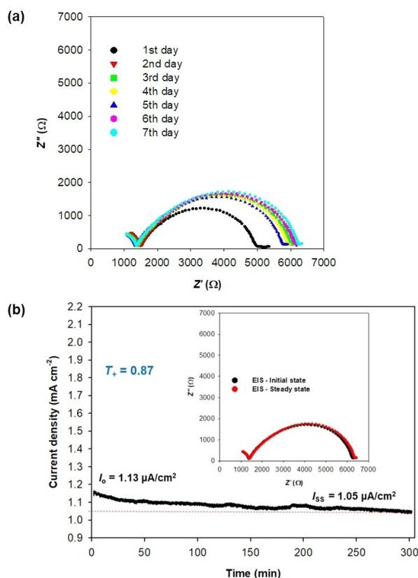
**Figure 6.** a) Interfacial resistances measured at different storage times and b) lithium transference number determination by potentiostatic polarization. Both samples are for the same symmetric Li/P(CL<sub>80</sub>TMC<sub>20</sub>)–LiTFSI<sub>0.28</sub>–ZrO<sub>2</sub>/Li cell and data were obtained at 21–22 °C.
