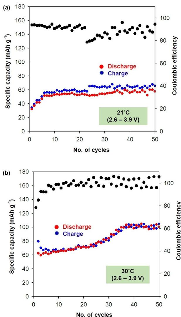
**Figure 8.** Charge-discharge galvanostatic profiles and coulombic efficiency of LFP half-cells using  $\text{P}(\text{CL}_{80}\text{TMC}_{20})\text{-LiTFSI}_{0.28}\text{-ZrO}_2$  (4 wt.%) electrolytes in potential ranges of (a) 2.6–3.9 V at 21 °C and (b) 2.6–3.9 V at 30 °C.
