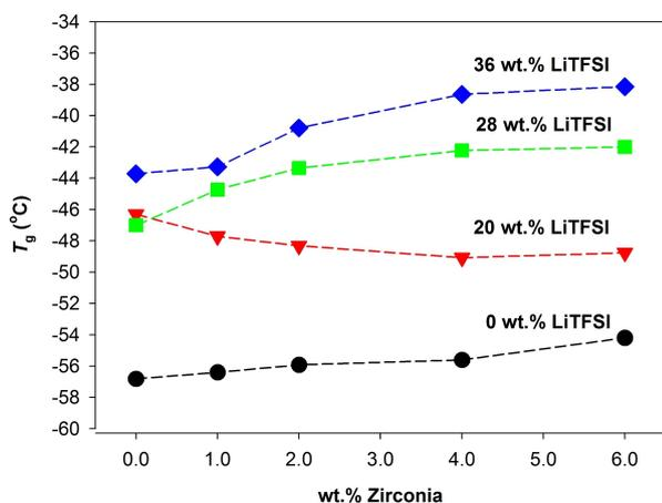
Figure 2.  $T_g$  vs wt.% of zirconia for P(CL<sub>80</sub>TMC<sub>20</sub>)–LiTFSI<sub>x</sub>–ZrO<sub>2</sub> samples.
