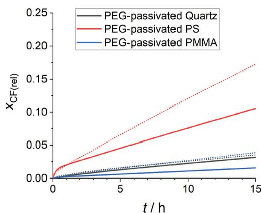
**Figure 5.** Spontaneous leakage of CF from POPC:chol liposomes containing POPC:chol with the molar composition 60:40 monitored in passivated quartz (black), passivated PS (red) and passivated PMMA (blue) cuvettes with a stirring rate of 300 (solid lines) and 900 (dotted lines) rpm.
