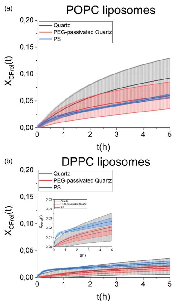
**Figure 9.** Spontaneous leakage of CF from (a) POPC and (b) DPPC liposomes monitored in quartz cuvettes (black), passivated quartz cuvettes (red) and PS cuvettes (blue) with a stirring rate of 300 rpm. The errors bars indicate the standard error of the mean.
