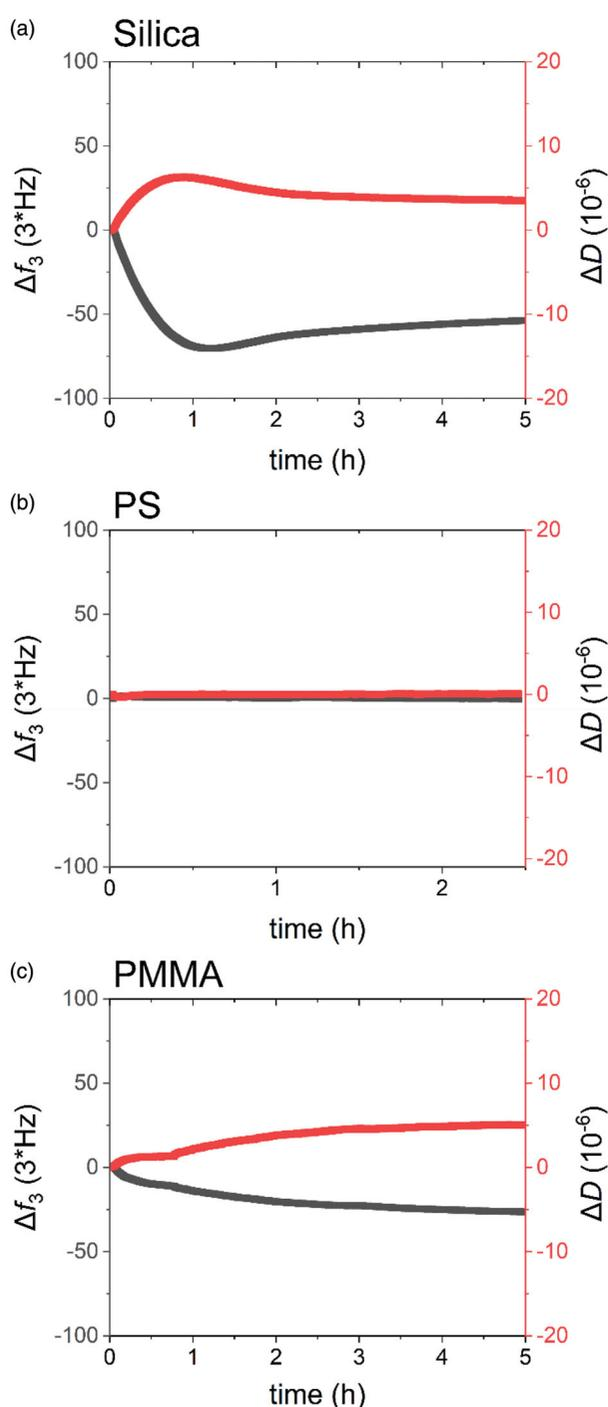
**Figure 2.** QCM-D recorded changes in frequency and dissipation upon interaction of POPC:chol liposomes with (a) silica (b) PS or (c) PMMA sensors.
