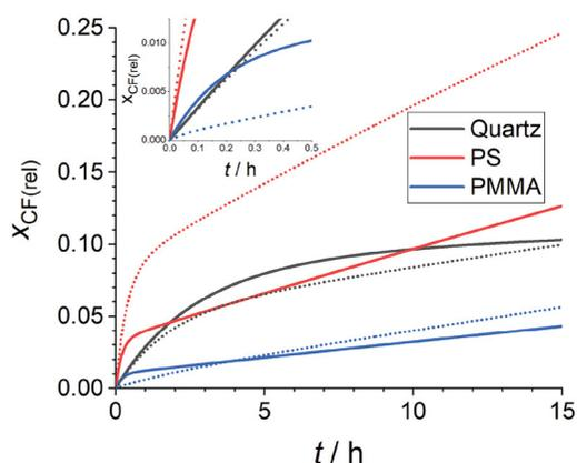
**Figure 1.** Spontaneous leakage of CF from POPC:chol (60:40) liposomes monitored in quartz (black), PS (red) and PMMA (blue) cuvettes with a stirring rate of 300 (solid lines) and 900 (dotted lines) rpm. The inset is highlighting the first half hour of the experiments.
