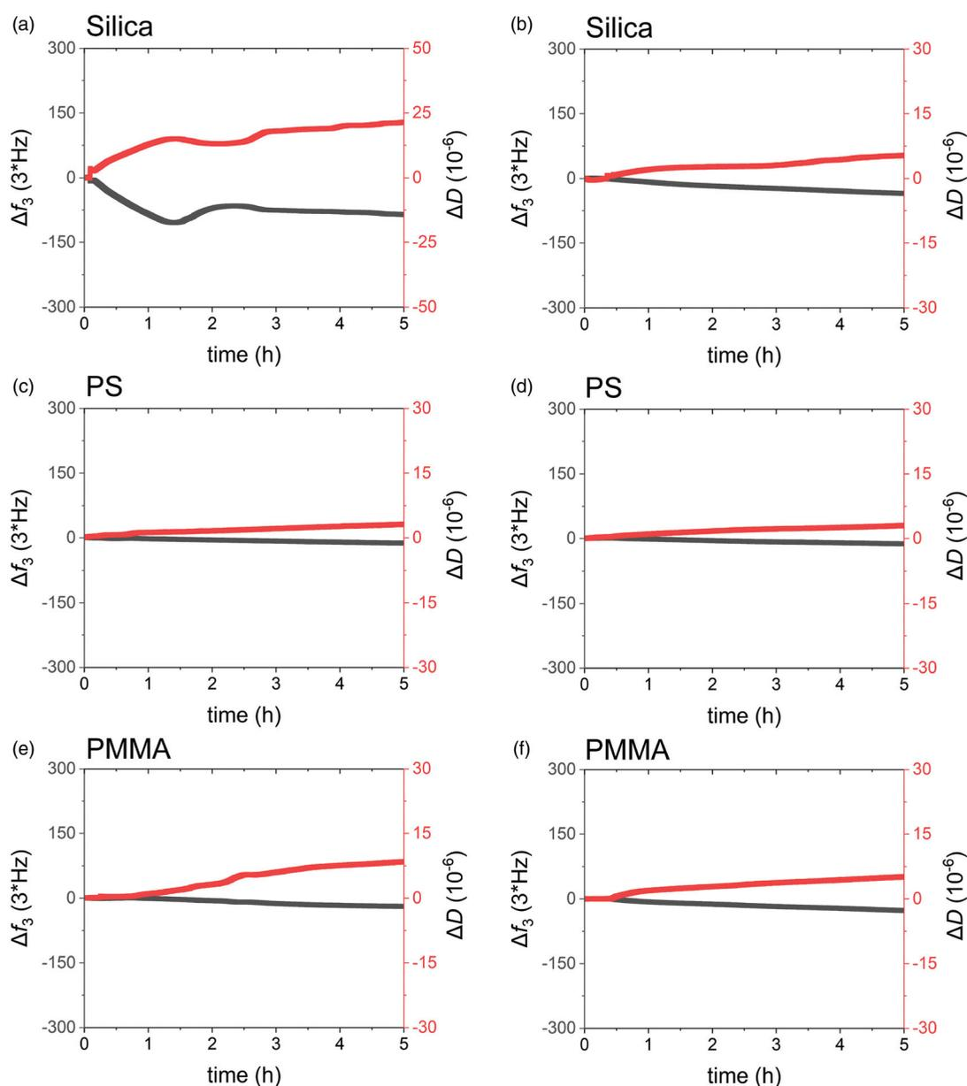
**Figure 4.** QCM-D graphs of POPC:chol:DSPE-PEG2000 and POPC:chol:ganglioside liposomes with a molar composition of 56:40:4. POPC:chol:DSPE-PEG2000 liposomes measured with different sensors (a) silica, (c) PS, and (e) PMMA and POPC:chol:ganglioside liposomes measured with (b) silica, (d) PS, and (f) PMMA sensors.
