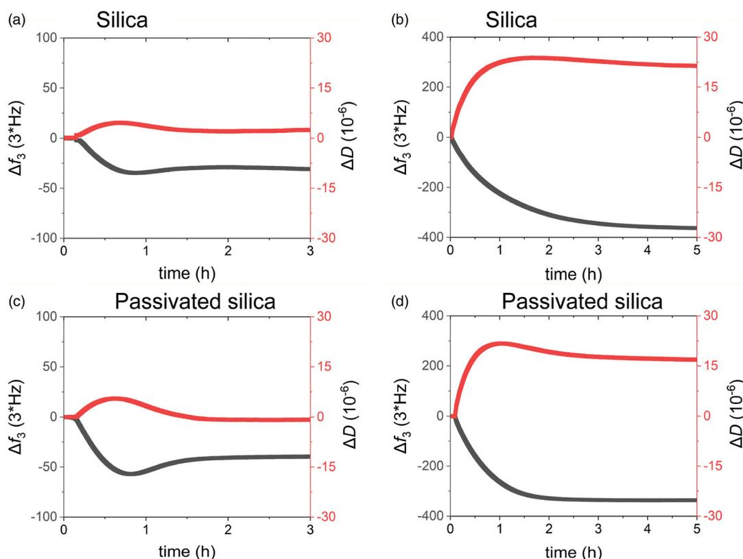
**Figure 10.** QCM-D graphs showing the interaction of POPC liposomes (left panel) and DPPC liposomes (right panel) with bare and PEG8000-passivated silica sensors.
