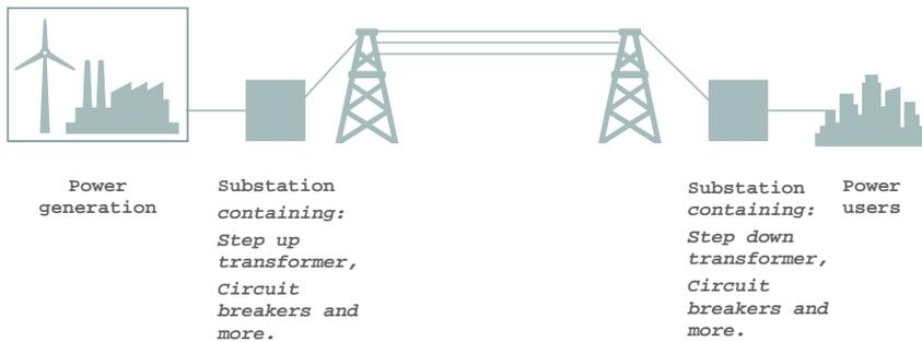
Figure 26: Very simplified picture of the power grid in which breakers and transformers are a part.
