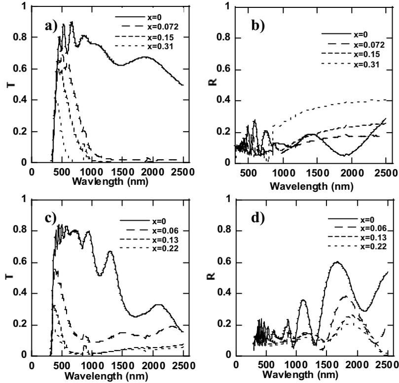
Fig. 5.5: Optical spectra in the wavelength range 300 – 2500 nm showing a) transmittance and b) reflectance of a Li-intercalated c-WO<sub>3</sub> film of thickness 460 nm, and c) transmittance and d) reflectance of a Li-intercalated a-WO<sub>3</sub> film of thickness 745 nm.
