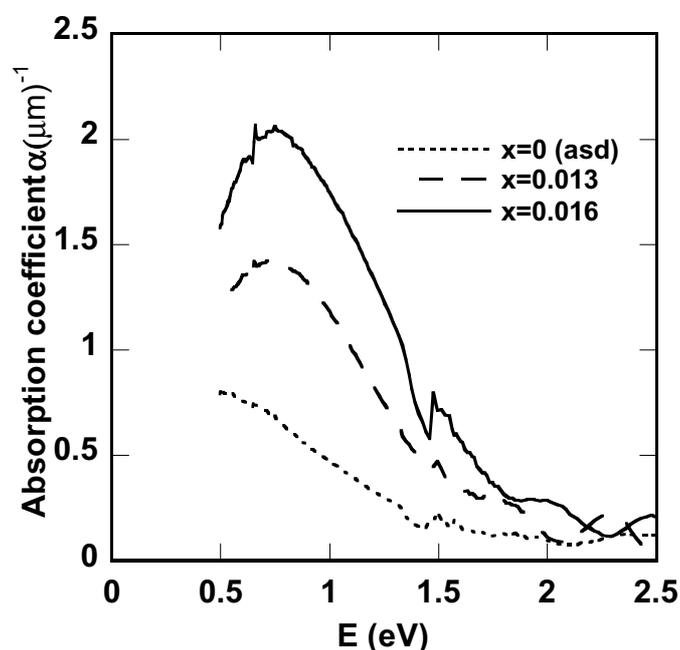
Fig. 5.6: Near-infrared absorption coefficient of  $c\text{-WO}_3$  films for the as-deposited state and at two low intercalation levels (given as Li/W ratios  $x$ ).
