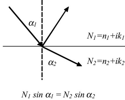
Fig. 2.4: Illustration of Snell's law of refraction at an interface between materials with refractive index  $N_1$  and  $N_2$ .
