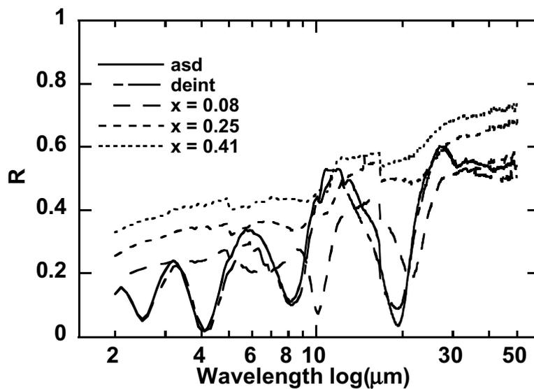
Fig. 5.2: Infrared reflectance of a 1450 nm thick c-WO<sub>3</sub> film, at different intercalation levels  $x$ , including the as-deposited (asd) and deintercalated (deint) states. The angle of incidence was 25°.
