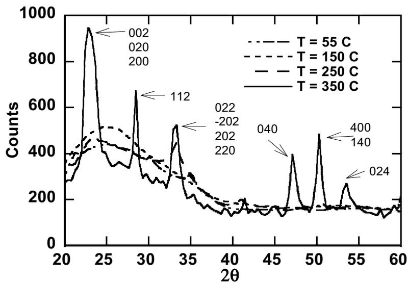
Fig. 4.2: X-ray diffractograms for monoclinic WO<sub>3</sub> sputtered at different substrate temperatures, shown in the figure. The indexed peaks are those of the monoclinic phase
