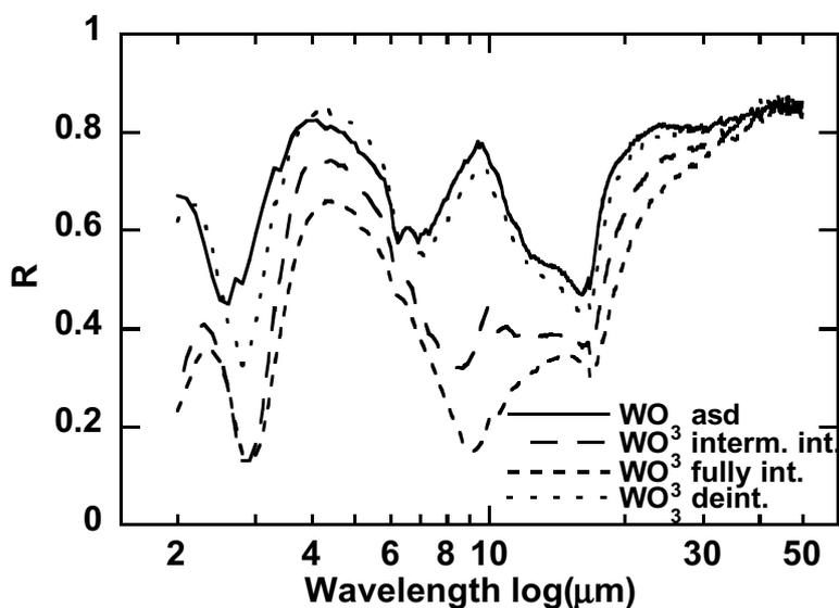
Fig. 5.9: Infrared reflectance spectra of an all-thin-film glass | ITO |  $\text{NiV}_x\text{O}_y\text{H}_z$  |  $\text{ZrO}_2$  | a- $\text{WO}_3$  | Al-grid device with a single layer of a- $\text{WO}_3$ . The spectra were taken when the a- $\text{WO}_3$  film was as-deposited, intermediately intercalated, fully intercalated and deintercalated, as specified in the figure. A voltage of  $-/+5$  V was applied at the Al grid during intercalation/deintercalation.
