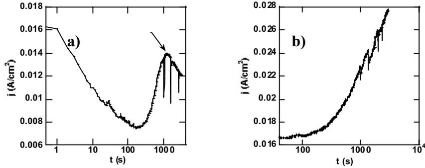
Fig. 5.11: Current densities during intercalation of an all-thin-film device with a) a-WO<sub>3</sub>, and b) c-WO<sub>3</sub>. The arrow in a) indicates when the ions have travelled to the Al contact. This feature is not seen in the device with c-WO<sub>3</sub> in b). A voltage of  $-/+5$  V was applied at the Al grid during intercalation/deintercalation.
