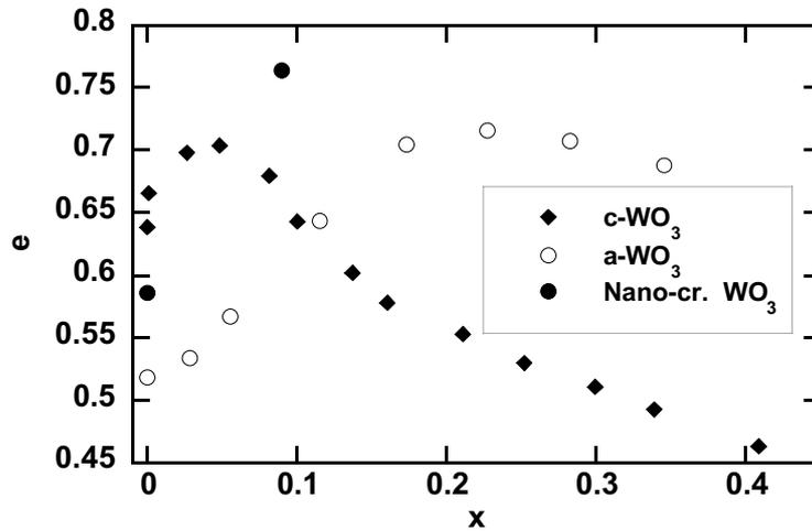
Fig. 5.4: Emittance calculated from reflectance spectra, for a c-WO<sub>3</sub> film of thickness 1270 nm, an a-WO<sub>3</sub> film of thickness 1450 nm and a nanocrystalline WO<sub>3</sub> film of thickness 2800 nm.
