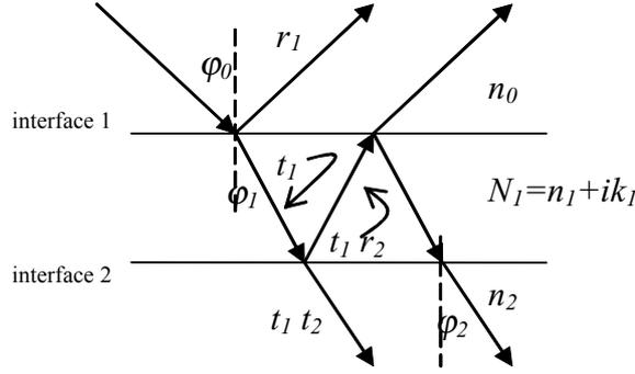
Fig. 2.5: Multiple reflections in a thin film layer of refractive index  $N_1$ , the angle of incidence is  $\varphi_0$ , the substrate refractive index is  $n_2$  and the refractive index of the ambient medium is  $n_0$ .
