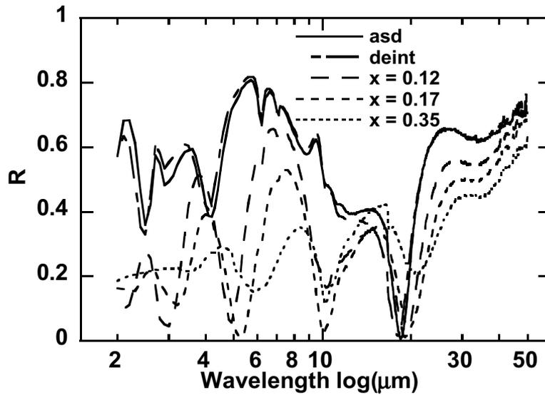
Fig. 5.1: Infrared reflectance of a 1270 nm thick a-WO<sub>3</sub> film at different intercalation levels  $x$ , including the as-deposited (asd) and deintercalated (deint) states. The angle of incidence was 25°.
