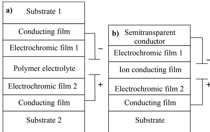
Fig. 2.1: The two basic configurations of electrochromic devices: a) is the conventional laminated device, and b) is the principle of the ATF device for IR-modulation.
