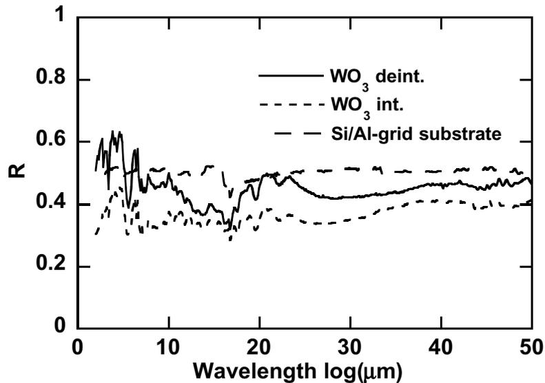
Fig. 5.7: Infrared reflectance spectra of a laminated glass | ITO |  $\text{NiV}_x\text{O}_y\text{H}_z$  | polymer | a- $\text{WO}_3$  | Al-grid | Si device with the  $\text{WO}_3$  film in intercalated and deintercalated states. The reflectance of the Si/Al-grid substrate is shown for comparison.
