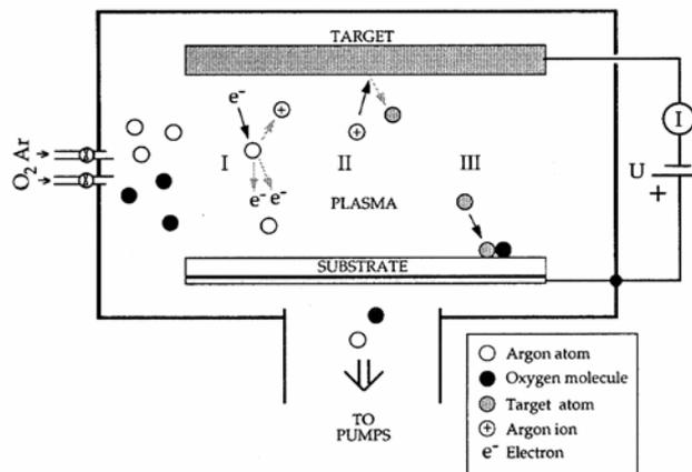
Fig. 4.1: Illustration of the DC glow discharge sputtering system. (After Veszelei<sup>59</sup>.)
