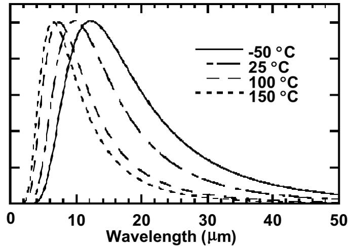
Fig. 2.3: The normalized blackbody spectra for different temperatures.
