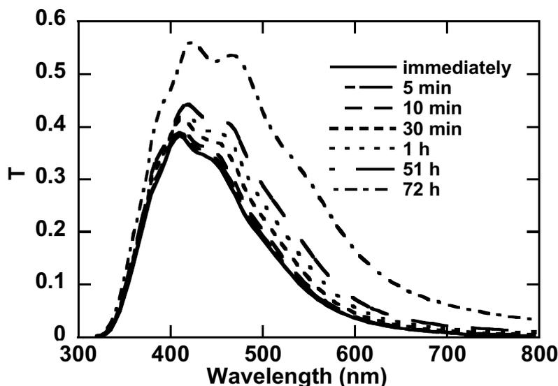
Fig. 4.4: Transmission loss due to leakage after certain elapsed times for an intercalated  $\text{WO}_3$  film.
