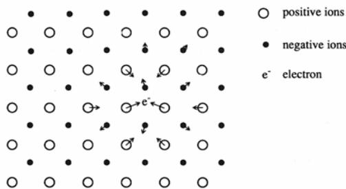
Fig. 2.6: The electron is trapped in the distorted lattice.(After Klingshim<sup>51</sup>)
