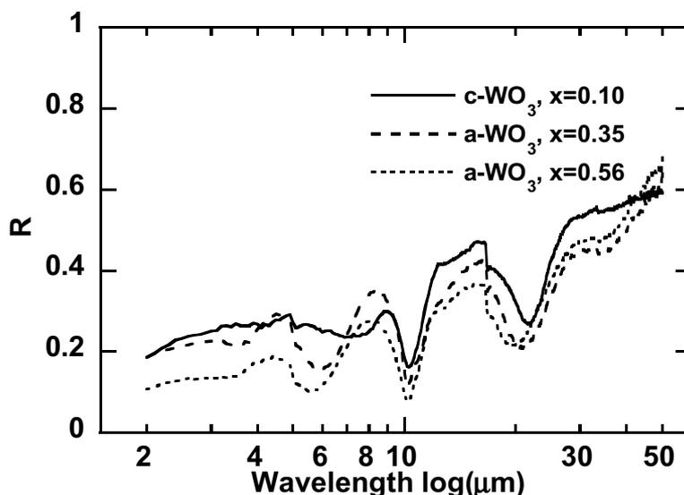
Fig. 5.3: Infrared reflectance of c-WO<sub>3</sub> and a-WO<sub>3</sub> films at the intercalation levels  $x = 0.10$  and  $0.35$ , as well as  $0.56$ , respectively. The films were the same as in Fig. 5.1 and Fig. 5.2.
