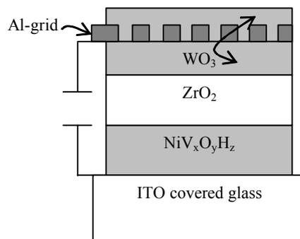
Fig. 5.8: Schematic sketch of the ATF III device with an embedded Al-grid.
