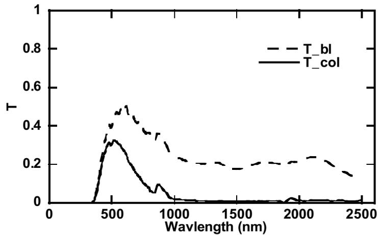
Fig. 5.12: Reflectance spectra in the range 0.3 – 2.5  $\mu\text{m}$ , of an all-thin-film glass | ITO |  $\text{NiV}_x\text{O}_y\text{H}_z$  |  $\text{ZrO}_2$  |  $\text{c-WO}_3$  | Al-grid |  $\text{c-WO}_3$  device with two layers of  $\text{c-WO}_3$  embedding the Al-grid. The spectra were taken when the  $\text{c-WO}_3$  film was bleached and coloured. A voltage of  $-/+5$  V was applied at the Al grid during intercalation/deintercalation.
