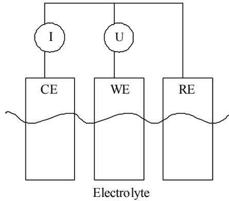
Fig. 4.3: Schematic picture of a three-electrode set-up with counter electrode (CE), working electrode (WE) and reference electrode (RE) in a liquid electrolyte.
