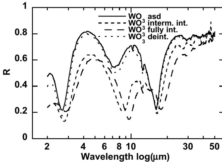
Fig. 5.10: Infrared reflectance spectra of an all-thin-film glass | ITO | NiV<sub>x</sub>O<sub>y</sub>H<sub>z</sub> | ZrO<sub>2</sub> | c-WO<sub>3</sub> | Al-grid device with a single layer of c-WO<sub>3</sub>. The spectra were taken when the WO<sub>3</sub> film was as-deposited, intermediately intercalated, fully intercalated and deintercalated, as given in the figure. A voltage of -/+5 V was applied at the Al grid during intercalation/deintercalation.
