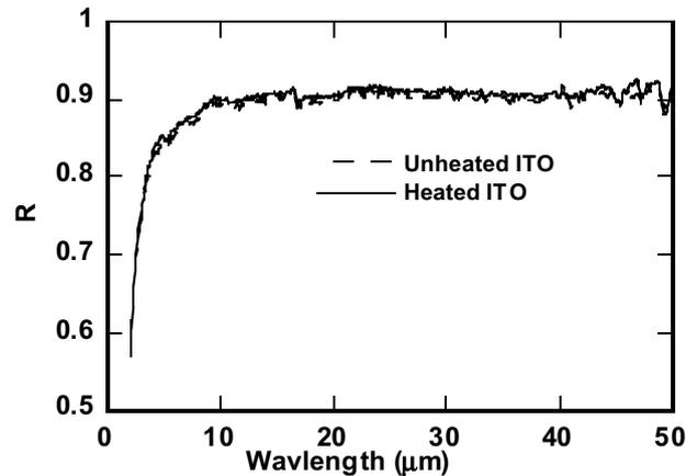
Fig. 2.2: Infrared reflectance spectra of an ITO film on glass that has been heated and an unheated reference sample.
