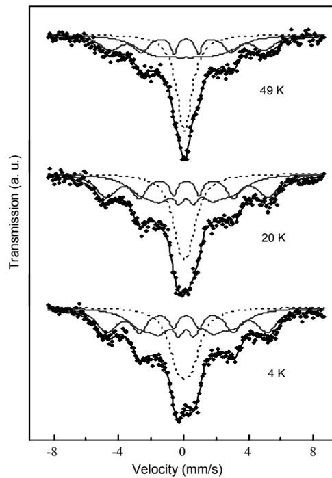
**Fig. 4.2.** Low temperature Mössbauer spectra of annealed MA  $\text{Fe}_{73}\text{Ni}_{27}$  alloy.
