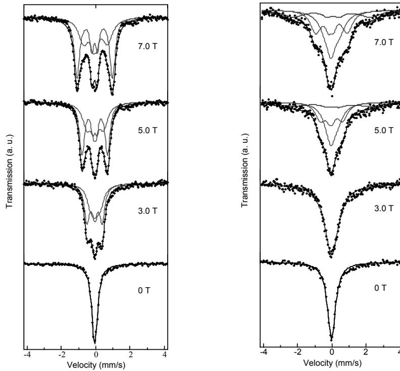
**Fig. 4.4.** RT Mössbauer spectra of the MA  $\gamma$  (fcc)  $\text{Fe}_{79}\text{Ni}_{21}$  alloy (left) and  $\text{Fe}_{73}\text{Ni}_{27}$  alloy (right) collected at different external fields applied parallel to the direction of the  $\gamma$ -ray.
