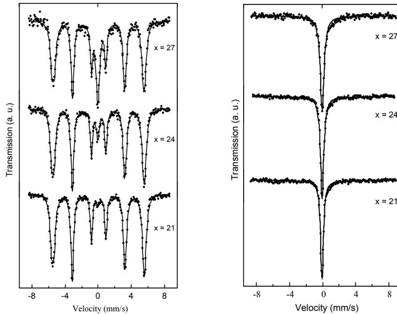
**Fig. 4.1.** RT Mössbauer spectra of MA  $\text{Fe}_{100-x}\text{Ni}_x$  ( $x = 21, 24,$  and  $27$  at %) alloys. Left: as-milled samples, sextet (bcc), singlet (fcc); right: after annealing at 650 °C.
