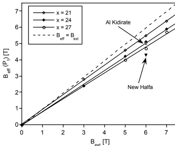
**Fig. 4.7.**  $B_{eff}(P_\gamma)$  vs.  $B_{ext}$  for MA  $\gamma$  (fcc)  $Fe_{100-x}Ni_x$  ( $x = 21, 24,$  and  $27$  at %) alloys. The data points for antitaenite from Al Kidirate and New Halfa meteorites at  $6.0$  T are also shown.
