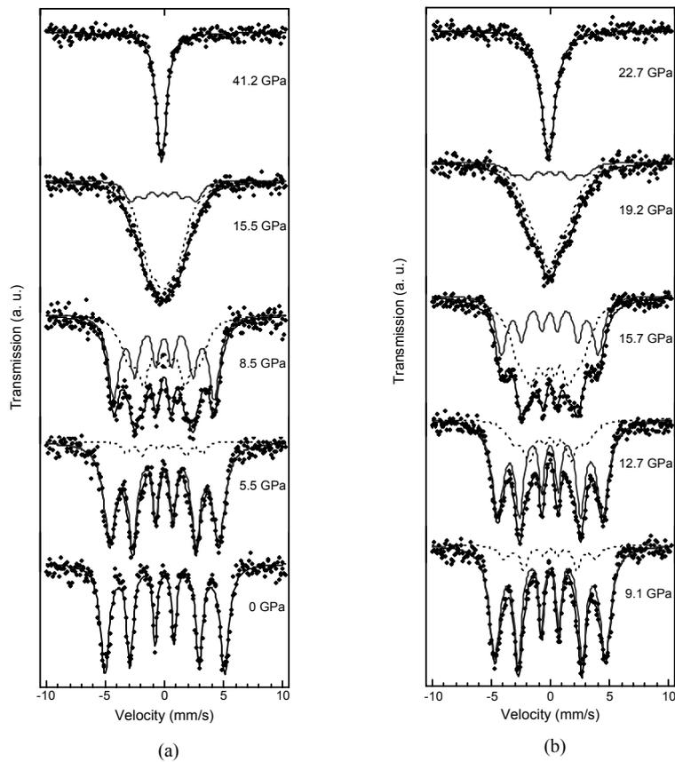
**Fig. 5.1.** High pressure Mössbauer spectra of  $^{57}\text{Fe}_{53}\text{Ni}_{47}$  alloy collected at RT: (a) compression; (b) decompression.
