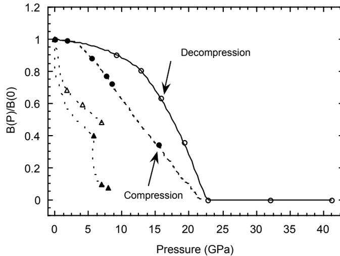
**Fig. 5.2.** Pressure dependence of the normalized weighted average hyperfine field for  $^{57}\text{Fe}_{53}\text{Ni}_{47}$  alloy: filled circles (compression), open circles (decompression). Open and filled triangles represent data from ref. [44] (at 4.2 K) for Invar  $\text{Fe}_{65}\text{Ni}_{35}$  and  $\text{Fe}_{68.5}\text{Ni}_{31.5}$ , respectively. The lines through the data points are only guides to the eye.
