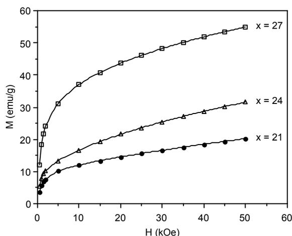
**Fig. 4.5.** Magnetization ( $M$  vs.  $H$ ) plots of the MA  $\gamma$  (fcc)  $Fe_{100-x}Ni_x$  ( $x = 21, 24,$  and  $27$  at %) alloys at 295 K.
