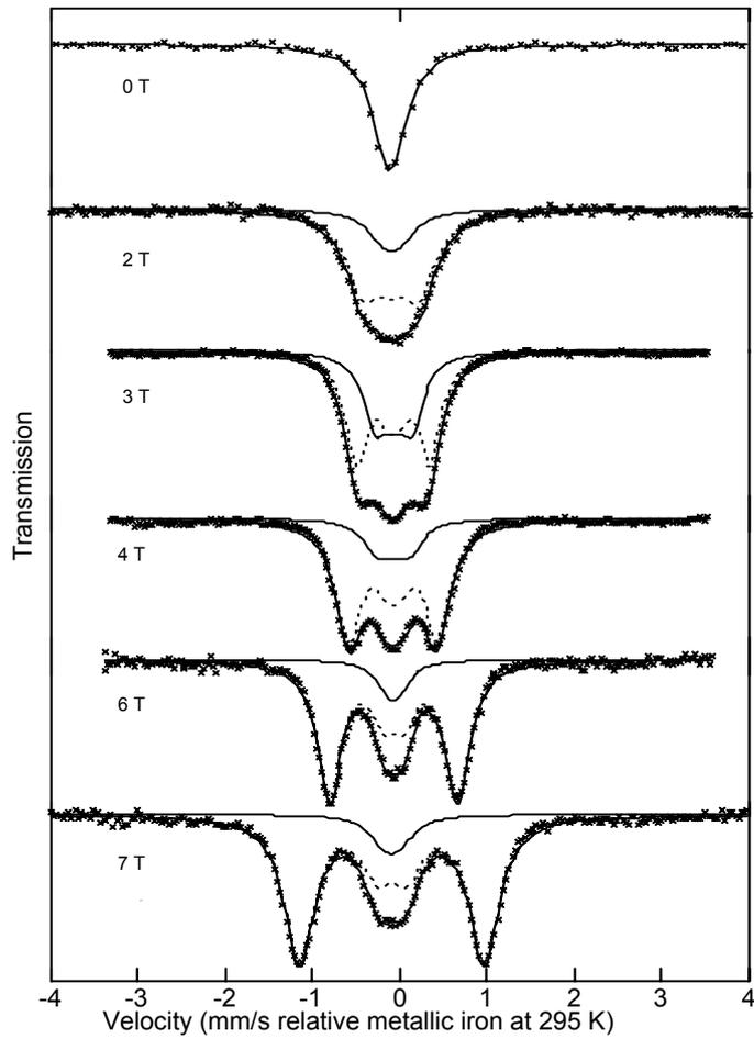
**Fig. 4.8.** Mössbauer spectra of the stainless steel  $Fe_{69}Cr_{18.5}Ni_{10.3}Mn_{1.8}$  foil recorded at room temperature in longitudinal external fields. The spectra are fitted using two quadruplets (lines 2 and 5 missing in an ordinary sextet). The high field (dashed line) and low field (full line) components are also shown.
