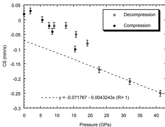
**Fig. 5.3.** Pressure dependence of the Mössbauer centre shift for  $^{57}\text{Fe}_{53}\text{Ni}_{47}$  alloy. The dashed line is a linear fit to the CS's above 20 GPa.
