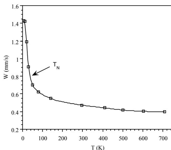
**Fig. 4.3.** Variation of the Mössbauer linewidth with temperature for the singlet subspectrum of annealed MA  $\text{Fe}_{76}\text{Ni}_{24}$  alloy. The line through the data points is only a guide to the eye.
