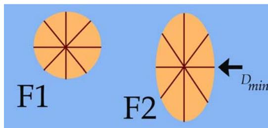
Figure 10. F1 shows a perfectly perpendicular cut fibre, where all diameters are the same. F2 shows an obliquely cut fibre. The minimum diameter ( $D_{min}$ ) is the same as the diameter if the fibre was perfectly perpendicular cut.
