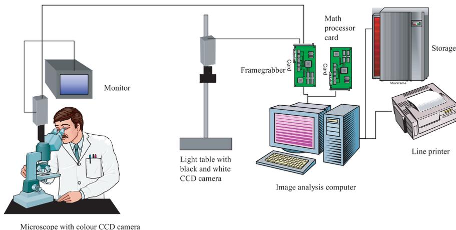
Figure 13. A schematic drawing of the image analysis setup.
