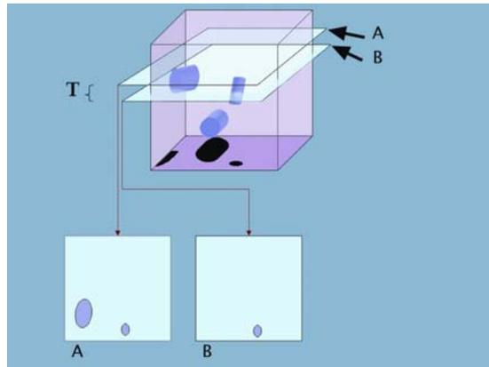
*Figure 1.* The disector principle. Two sections (planes) are placed in a volume a known distance apart ( $T$ ). Objects in the volume will be seen as profiles on the slices. The big object to the right is seen on slice S1 but not on S2 and are therefore counted. The smaller object to the left is seen on both slices. It is not counted yet. It will be counted on the slice before it disappears.
