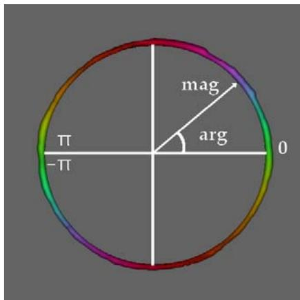
*Figure 2.* The GOP<sup>®</sup> circle. A special colour scheme is used for the angle, or argument ( $\text{arg}$ ), of the vector. The length of the vector, the magnitude ( $\text{mag}$ ), depends on the strength of the feature analysed.
