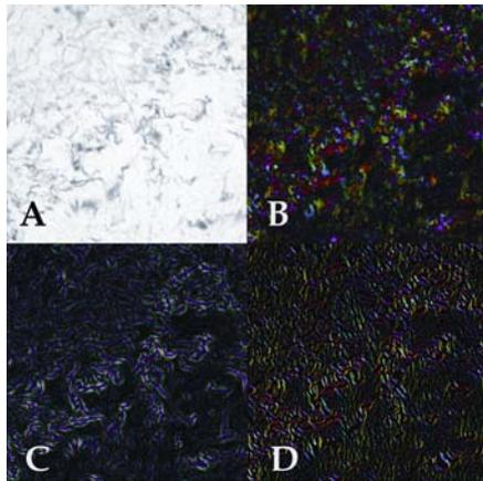
*Figure 4.* (a). The same operations as in fig. 3 are performed on a specimen consisting of elastic fibres (black and white image). In (b) the Orient operation is shown, in (c) the phase operation and in (d) the line operation.
