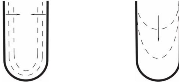
Figure 3. Origin of hysteresis between adsorption (left) and desorption (right) curves.
