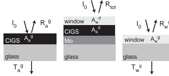
Figure 2.19: Samples and measurements used for estimating the absorptance in the absorber layer with the method used in Paper III. A_a^d(\lambda) is the desired CIGS absorber absorptance of the complete device structure in the middle, A_w^d is the absorptance of the ZnO:Al/ZnO/CdS window layers in the device, and R_{tot} is the measured total reflectance of the device. R_a^g , T_a^g , and A_a^g denote the reflectance, transmittance and absorber absorptance for the absorber/glass substrate structure to the left, and R_w^g , T_w^g , and A_w^g are the corresponding quantities for the window/glass substrate structure to the right.
