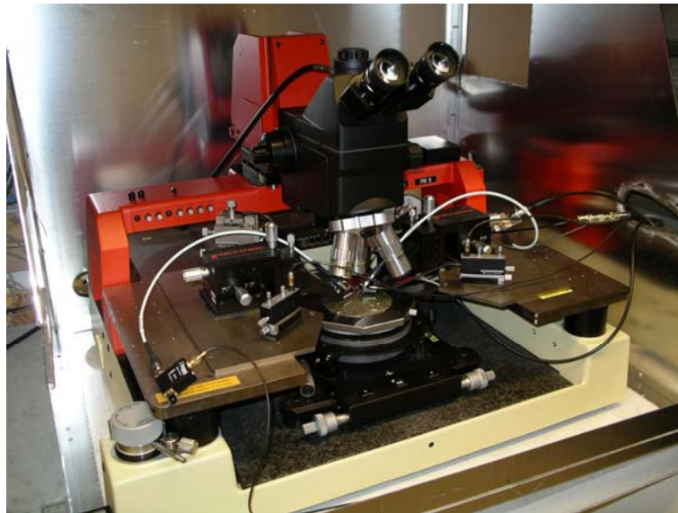
Figure 14. Probe station for high-frequency on-wafer measurements.
