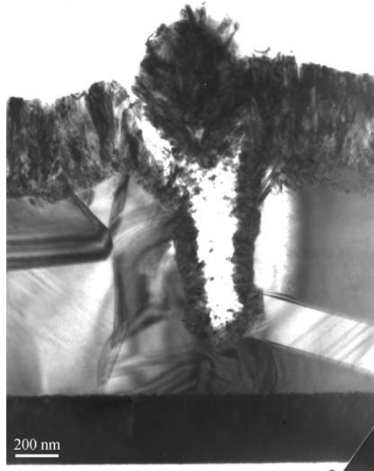
Figure 2.3: Transmission electron micrograph of a deep trench in a CIGS film uniformly covered by ALD-ZnO. The top layer of sputtered ZnO does not cover the trench.
