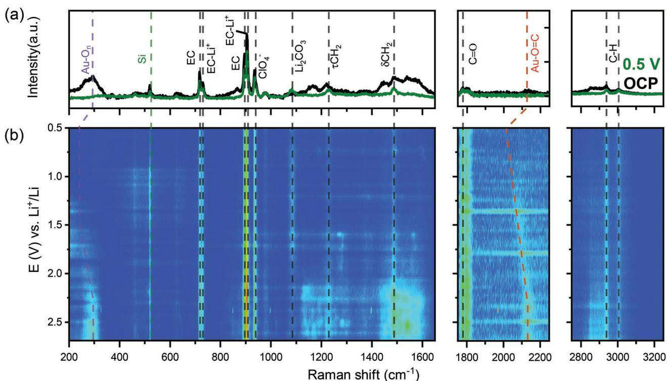
**Figure 2.** a) Raman spectra at OCP (black) and 0.5 V (green) and b) Contour plot showing operando Raman spectra during the first reduction half cycle of an Au SERS substrate used as working electrode in  $\text{LiClO}_4/\text{EC}$ .
