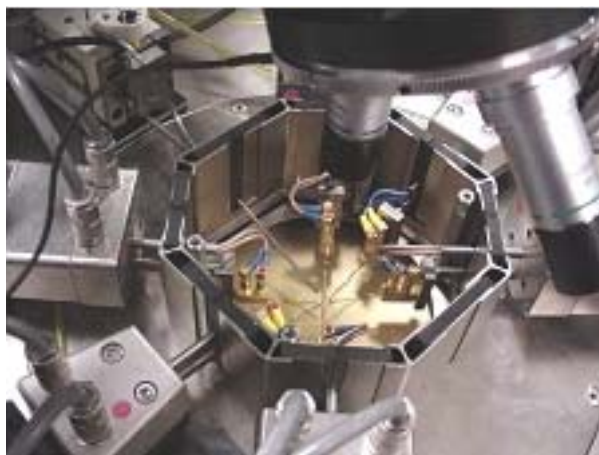
Figure 6.8: The shielded micro-chamber on a Cascade Summit 12k used to protect the DUT (device under test) from EMC disturbances.
