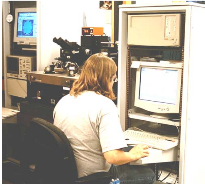
Figure 6.1: The author of this thesis is working with the Keithley 4200-SCS parameter analyzer at Philips Research/Eindhoven. In the background the Cascade 12k Summit semi-automatic probe-station is visible, and on the monitor in the background is a wafer map shown. This system was used in Paper III and Paper IV.
