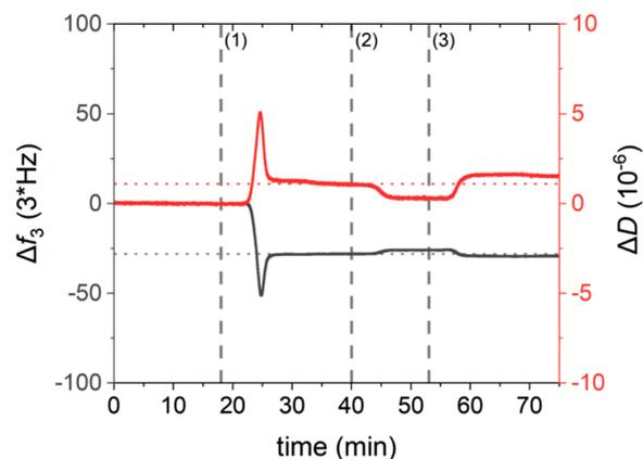
Fig. 1. QCM-D measurement of silica sensor (1) interacting with a solution containing POPC-liposomes, forming a POPC-SLB; (2) as the sensor was then rinsed with a buffer solution; (3) as a fresh batch of POPC-liposomes is inserted into the system. Changes in frequency (grey line) and dissipation (red line) were investigated.
