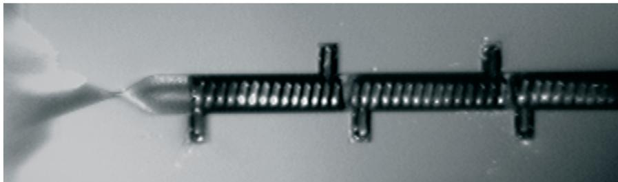
Figure 16. DLC heater elements integrated in a micro nozzle (The gas flow is from right to left)
